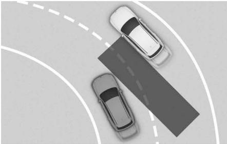
Blind-Spot Collision-Avoidance Assist may not detect a vehicle in an adjacent lane when driving on curves and may not activate a warning or brake your vehicle.
