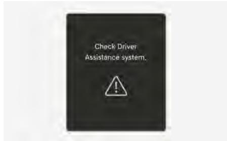
When Parking Collision-Avoidance Assist or other related functions does not work properly, the "**Check Driver Assistance system.**" warning message may appear on the instrument cluster, and Parking Collision-Avoidance Assist turns off automatically. Have your vehicle inspected by an authorized retailer of Genesis Branded products.
