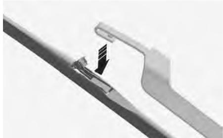
6. Install the new wiper blade assembly in the reverse order of removal.
