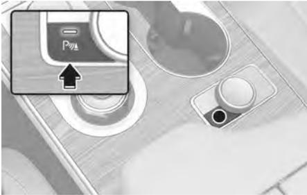
Press the Parking Safety (PWA) button to turn on Parking Distance Warning. Press the button again to turn off the function.
