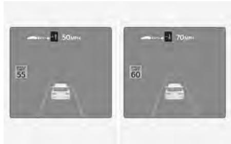
If the speed limit changes when using Manual Speed Limit Assist or Smart Cruise Control, an arrow in the direction of up or down appears to inform you to change the set speed by pushing the **+** or **-** switch.
