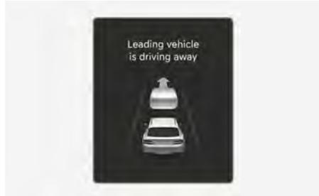
When a detected vehicle in front departs from a stop, Leading Vehicle Departure Alert displays the "**Leading vehicle is driving away**" message on the instrument cluster and an audible warning sounds.
