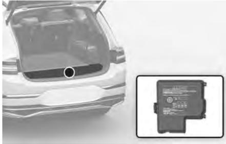
Inside the fuse panel cover, you can find the panel label describing fuse names and ratings.
