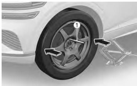
13. Tighten the wheel bolts with your fingers onto the studs with the smaller end of the wheel bolts closest to the wheel.
