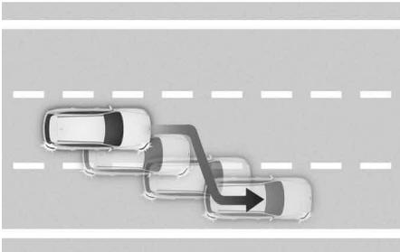
Highway Lane Change Assist function helps change lanes to the direction you operate the turn signal switch if the function judges that lane change is possible.
