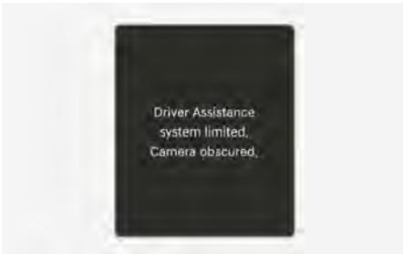
If the front view camera or front radar is covered or blocked, its detecting performance is reduced, and Lane Keeping Assist may be temporarily limited or disabled.
