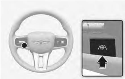
With the engine on, press and hold the Lane Driving Assist (/👁) button located on the steering wheel to turn on and off. When Lane Keeping Assist is on, the /👁 indicator is on.
