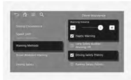
With the engine on, select **Setup** > **Vehicle** > **Driver Assistance** > **Warning Methods** from the Settings menu in the infotainment system to select the following:
