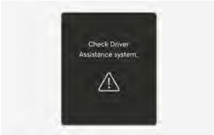
When Rear Cross-Traffic Collision-Avoidance Assist is not working properly, the "**Check Driver Assistance system**" warning message may appear for several seconds, and the
