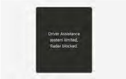
If the rear corner radar is blocked or covered, or when the rear bumper around the rear corner radar or sensor is covered by any foreign material, such as snow, rain, or dirt, or when a trailer or hitch mounted carrier is installed, the detecting performance may decrease and temporarily limit or disable Safe Exit Assist.
