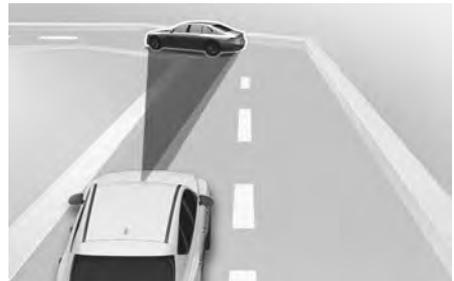
On curves, Smart Cruise Control may not detect a vehicle in the same lane, and may accelerate to the set speed. Your vehicle speed may be reduced if a vehicle is detected in an adjacent lane and your vehicle speed may rapidly decrease when a vehicle ahead is detected suddenly.
