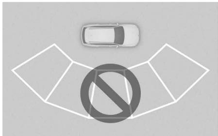
Remote Smart Parking Assist does not work normally when the parking lines are not parallel. Do not park even though the parking space is recognized by the sensor.
