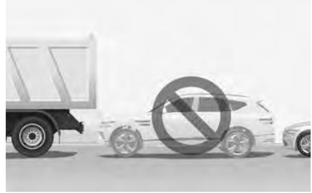
Do not use Remote Smart Parking Assist around vehicles with higher ground clearance, such as a bus, truck, etc. It may lead to an accident.
