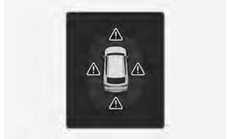
When the Parking Collision-Avoidance Assist Warning is operating, if the function is not working normally or the ultrasonic sensor is blocked, the
