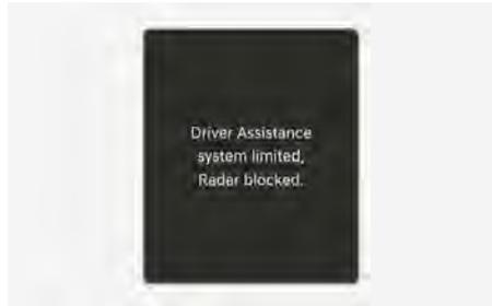
If the rear corner radar is blocked or covered, or when the rear bumper around the rear corner radar or sensor is covered by any foreign material, such as snow, rain, or dirt, or when a trailer or hitch mounted carrier is installed, the detecting performance may reduce and temporarily limit or disable Blind-Spot Collision-Avoidance Assist.
