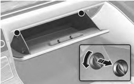
3. Press and hold the lock on the left side of the cover.
