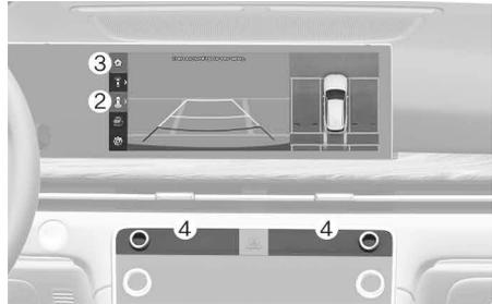
The rear view appears on the screen to assist parking. The rear view has top view, rear view, side view, and 3D view.
