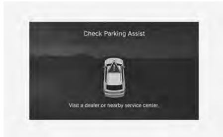
When Remote Smart Parking Assist is not working properly, the Check Parking Assist warning message may appear on the infotainment system screen. If the message appears, stop using Remote Smart Parking Assist, and have your vehicle inspected by an authorized retailer of Genesis Branded products.
