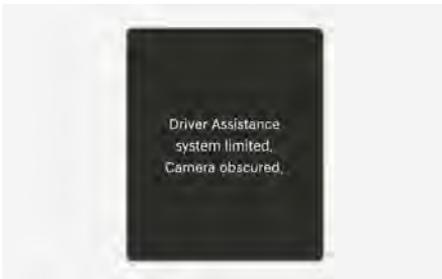
If the front view camera is covered or blocked, its detecting performance is reduced, and Driver Attention Warning may be temporarily limited or disabled.
