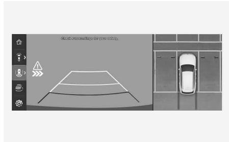
To warn you of an approaching vehicle from the rear left or right of your vehicle, the warning light on the side view mirror may blink, a warning message may appear on the instrument cluster, an audible warning may sound, and the steering wheel may vibrate.
