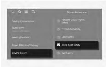
With the engine on, select **Setup** > **Vehicle** > **Driver Assistance** > **Driving Safety** from the Settings menu to select the following:
