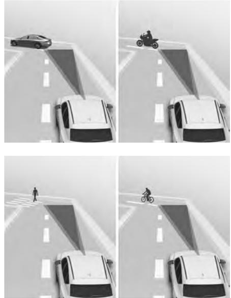
Forward Collision-Avoidance Assist may not detect other vehicles, powered two-wheelers, pedestrians, or cyclists in front of you when driving on a curve adversely affecting the performance of the sensors. A warning, brake assist, or steering assist (if equipped) may not be activated when needed.
