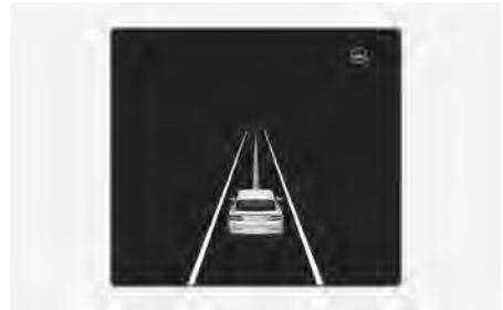
If the both lane markings and/or vehicle ahead are detected and your vehicle speed is below 124 mph (200 km/h), the green Ⓢ indicator light illuminates on the instrument cluster, and Lane Following Assist helps center the vehicle in the lane by assisting the steering wheel.
