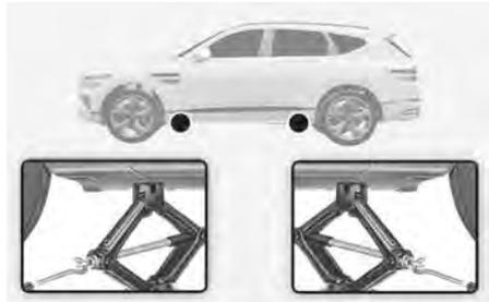
8. Insert the jack handle into the jack and turn it clockwise, raising the vehicle until the tire clears the ground. Make sure the vehicle is stable on the jack.
