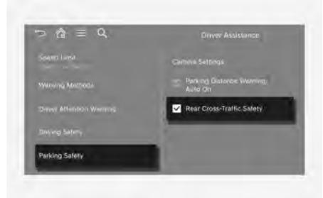
With the engine on, select **Setup > Vehicle > Driver Assistance > Parking Safety > Rear Cross-Traffic Safety** from the Settings menu in the infotainment system to turn on Rear Cross-Traffic Collision-Avoidance Assist and deselect to turn off the function.
