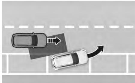
Blind-Spot Collision-Avoidance Assist may brake your vehicle if there is a detected collision risk in the blind spot area when driving forward out of a parking space.
