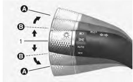
Highway Lane Change Assist function operates, when you push the turn signal lever up or down to the [A] or [B] position while the function is in the ready state (indicator is green), and all of the following conditions are met:
