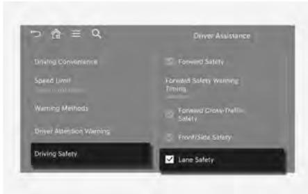
With the engine on, select **Setup > Vehicle > Driver Assistance > Driving Safety** from the Settings menu in the infotainment system to select the following:
