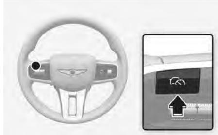
Press the Driving Assist (DRIVING ASSIST) button to turn off Manual Speed Limit Assist. The Speed Limit (SPEED LIMIT) indicator off.
