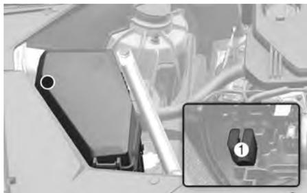
6. Check the removed fuse and replace it if it is blown. Spare fuses are provided in the instrument panel fuse panels (or in the engine compartment fuse panel).
