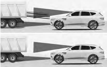
Forward Collision-Avoidance Assist may not be able to detect all potential hazards, like if the vehicle in front of you has cargo that extends rearward past the end of the vehicle or if the vehicle in front of you has higher ground clearance. Always maintain a safe distance from the vehicles ahead. Adjust your vehicle speed or steer your vehicle depending on the road conditions.
