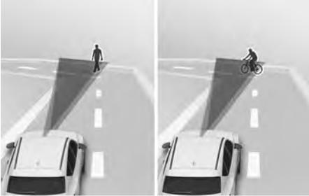
If a vehicle, powered two-wheeler, pedestrian, or cyclist is detected in the next lane or outside the lane when driving on a curve. Forward Collision-Avoidance Assist may warn you and may brake or steer (if equipped) your vehicle even when not needed.
