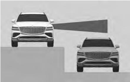
Blind-Spot Collision-Avoidance Assist may not operate properly when driving where the heights of the lanes are different. The system may not detect a vehicle on a road with a different lane height (underpass joining section, grade separated intersections, etc.) and not activate a warning or brake your vehicle.
