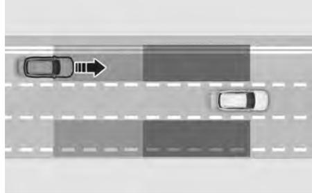
Blind-Spot Collision-Avoidance Assist helps detect and warns you that a vehicle is approaching at high speed from the blind spot area.
