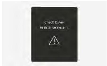
When Intelligent Speed Limit Assist is not working properly, the "**Check Driver Assistance system**" warning message may appear on the instrument cluster for several seconds, and the **!** and **☐** warning lights may illuminate on the instrument cluster. Have your vehicle inspected by an authorized retailer of Genesis Branded products.
