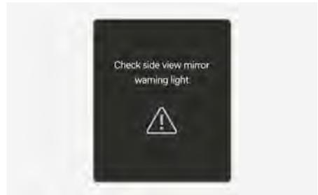
When the side view mirror warning light is not working properly, the "**Check side view mirror warning light.**" warning message may appear for several seconds, and the
