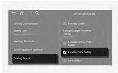
With the engine on, select or deselect **Setup** > **Vehicle** > **Driver Assistance** > **Driving Safety** > **Forward/Side Safety** from the Settings menu to turn on Lane-Change Oncoming function, Lane-Change Side function, and Evasive Steering Assist function.
