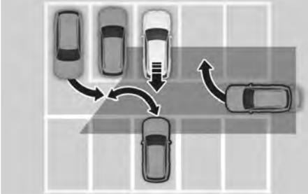
Rear Cross-Traffic Collision-Avoidance Assist may detect vehicles that are parking or pulling out near your vehicle (e.g. leaving beside your vehicle, parking or pulling out behind your vehicle, approaching your vehicle making a turn). If this occurs, the function may activate a warning and brake your vehicle even when not needed.
