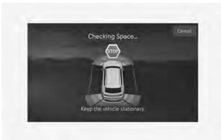
1. When the vehicle is stopped by depressing the brake pedal, the vehicle sensors detect the distance from nearby objects and check for space to exit.
