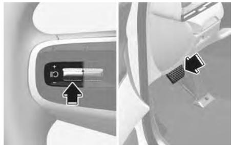
Press the || switch or depress the brake pedal to temporarily cancel Smart Cruise Control.
