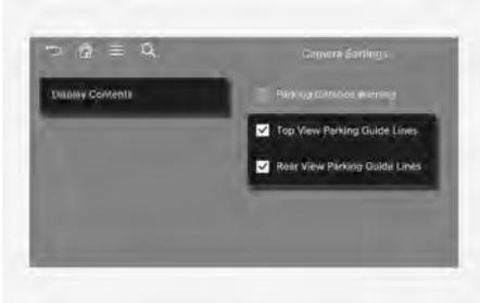
To change the settings of Surround View Monitor's display contents, press the setup icon (⚙️) on the screen while Surround View Monitor is operating, or select **Setup > Vehicle > Driver Assistance > Parking Safety > Camera Settings** from the Settings menu in the infotainment system while the engine is on.
