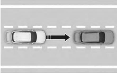
Highway Driving Assist helps maintain distance from the vehicle ahead, maintain the set speed, and center the vehicle in the lane while driving on the highway.
