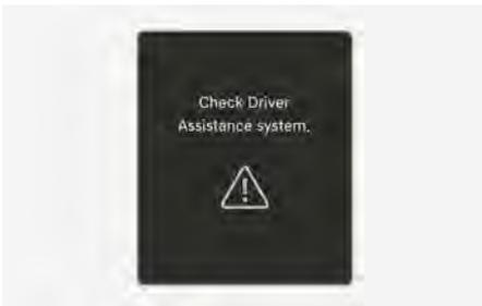
When Blind-Spot Collision-Avoidance Assist is not working properly, the "**Check Driver Assistance system**" warning message may appear for several seconds, and the ⚠ warning light may illuminate on the instrument cluster. Have your vehicle inspected by an authorized retailer of Genesis Branded products.
