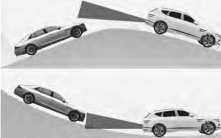
Blind-Spot Collision-Avoidance Assist may not detect a vehicle in an adjacent lane when the road merges or divides, and may not activate a warning or brake your vehicle.
