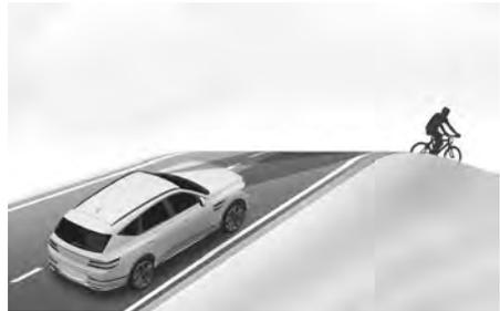
Forward Collision-Avoidance Assist may not detect other vehicles, powered two-wheelers, pedestrians, or cyclists in front of you while driving uphill or downhill, adversely affecting the performance of the sensors. A warning, brake assist, or steering assist (if equipped) may not be activated when needed.
