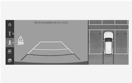
To warn you of an approaching vehicle from the rear left or right of your vehicle, the warning light on the side view mirror may blink, a warning message may appear on the instrument cluster, an audible warning may sound, and the steering wheel may vibrate.
