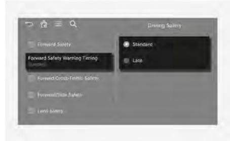
With the engine on, select **Setup > Vehicle > Driver Assistance > Driving Safety > Forward Safety Warning Timing** from the Settings menu in the infotainment system to change the initial warning activation time for Forward Collision-Avoidance Assist. The warning time can be set to either **Standard** (or **Normal**) or **Late**.
