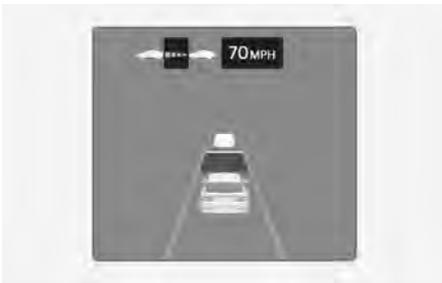
If you depress the accelerator pedal above a certain speed while Smart Cruise Control is operating, your vehicle can speed up temporarily without changing the set speed. The set speed, distance level, and target distance blink on the instrument cluster while depressing the accelerator pedal. Your vehicle speed may decrease if the accelerator pedal is not depressed far enough.
