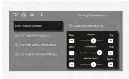
With the engine on, select **Setup > Vehicle > Driver Assistance > Driving Convenience > Smart Cruise Control** from the Settings menu in the infotainment system to adjust **Distance**, **Acceleration**, and **Response Speed** manually.
