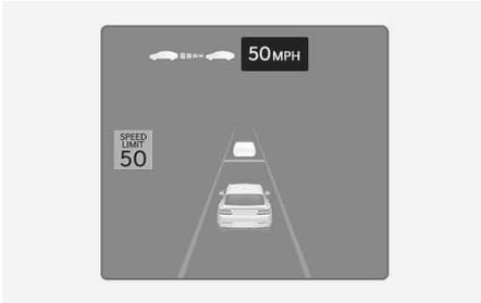
Manual Speed Limit Assist or Smart Cruise Control assists you to adjust the vehicle speed according to the speed limit. When the set speed is same as the speed limit, the set speed automatically changes to the current speed limit if the speed limit changes. The function operates on the road which has a speed limit of 44 mph (70 km/h) or higher. When the function is active, the set speed on the instrument cluster appears in green.
