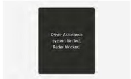
If the front radar is covered or blocked, its detecting performance is reduced, and Smart Cruise Control is temporarily limited or disabled.
