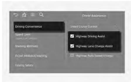
With the vehicle on, select or deselect **Setup > Vehicle > Driver Assistance > Driving Convenience** from the Settings menu to turn each function on and off.
