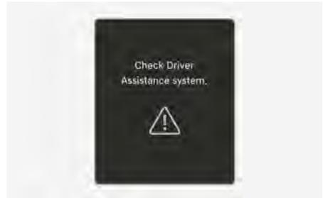
When Lane Following Assist is not working properly, the "**Check Driver Assistance system**" warning message may appear for several seconds, and the
