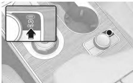
When the system is deactivated, the ISG OFF (A) button indicator illuminates and the message, **"Auto Stop is off. Shift to P or N to start engine manually"** appears on the cluster display with a warning sound.
