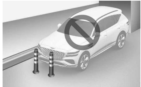
Remote Smart Parking Assist performance may be reduced or collided with an obstacle may occur when there is a narrow object, circular pillar, square pillar, or a pillar surrounded by objects such as a fire extinguisher, etc., near the parking space. Park or exit your vehicle manually.
