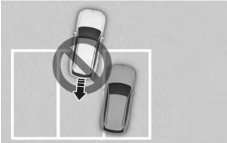
If Remote Smart Parking Assist is used, when parking next to a misaligned vehicle, your vehicle may cross the parking marking on the opposite side of the parked vehicle.
