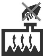
Never remove the engine coolant cap and/or liquid-cooled intercooler coolant cap or the drain plug while the engine coolant cap and liquid-cooled intercooler coolant cap are hot. Hot coolant and steam may blow out under pressure, causing serious injury.
