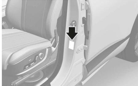
All specifications (sizes and pressures) can be found on a label attached to the driver's side center pillar.
