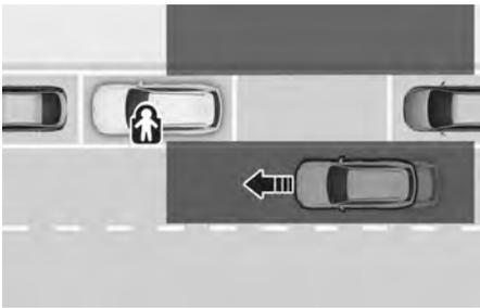
Safe Exit Assist helps detect a vehicle approach the rear corner of your vehicle, after the vehicle is stopped and a passenger opens a door.
