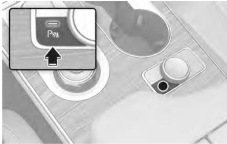
Press and hold the Parking Safety (PWA) button more than 2 seconds, to turn the Parking Collision-Avoidance Assist on or off.
