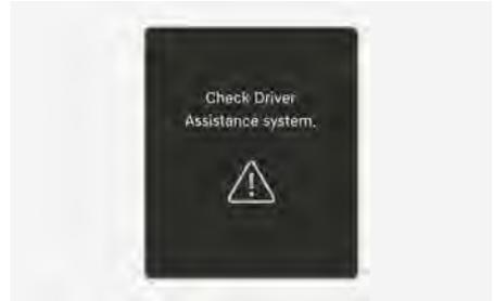
When Forward Collision-Avoidance Assist is not working properly, the "**Check Driver Assistance system.**" warning message may appear, and the ⚠, 🚲, and 🛵 warning lights illuminate on the cluster. Have your vehicle inspected by an authorized retailer of Genesis Branded products.
