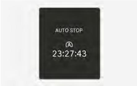
AUTO STOP display shows the elapsed time of engine stop by the Idle Stop and Go system.
