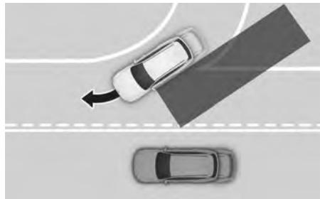
Blind-Spot Collision-Avoidance Assist may not detect a vehicle in an adjacent lane or may incorrectly detect the ground or another object when driving on hills and activate a warning or brake your vehicle.
