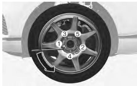
**Check the tire pressure after installing the compact spare tire. The compact spare tire should be inflated to 420 kPa (60 psi).**
