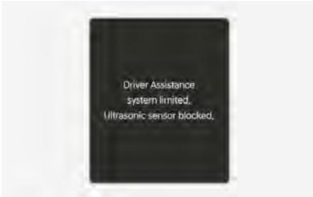
If the ultrasonic sensor is blocked or covered by any foreign material, such as snow, rain, or dirt, the detecting performance may reduce and temporarily limit or disable Parking Distance Warning.
