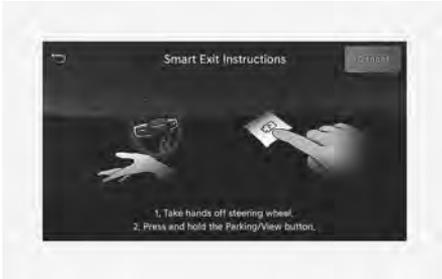
1. Press the Parking/View (**P**) button when the vehicle is stopped by depressing the brake pedal. When the brake pedal is released, Remote Smart Parking Assist automatically controls the steering wheel, vehicle speed, and gearshift.
