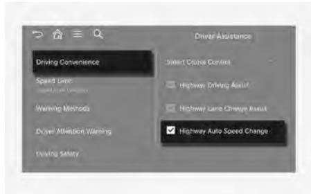
With the vehicle on, select **Setup > Vehicle > Driver Assistance > Driving Convenience > Highway Auto Speed Change** from the Settings menu in the infotainment system to turn on Navigation-based Smart Cruise Control and deselect to turn off the function.
