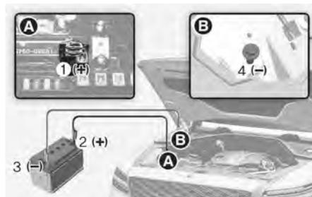
7. Connect the jumper cables in the exact sequence shown in the illustration. First connect one jumper cable to the positive (+) jumper terminal of your vehicle (1).
