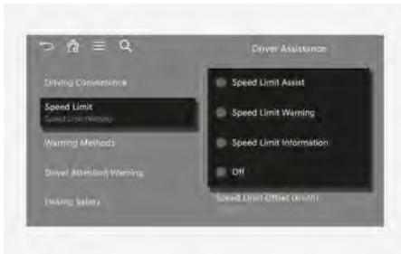
With the engine on, select **Setup > Vehicle > Driver Assistance > Speed Limit** from the Settings menu in the infotainment system to select the following:
