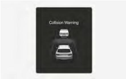
While Smart Cruise Control is operating and the collision risk of the vehicle ahead is high, the **"Collision Warning"** warning message appears on the instrument cluster, an audible warning sounds, and the steering wheel vibrates (if equipped).
