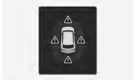
When the Parking Distance Warning is operating, if the function is not working normally or the ultrasonic sensor is blocked, the
