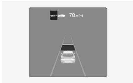
When Based on driving style is operating, the vehicle distance level and target distance appears white based on the driving style.
