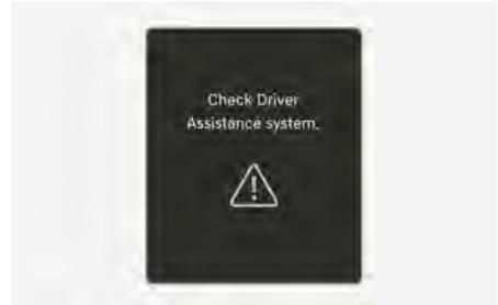
When Safe Exit Assist is not working properly, the "**Check Driver Assistance system.**" warning message may appear for several seconds, and the
