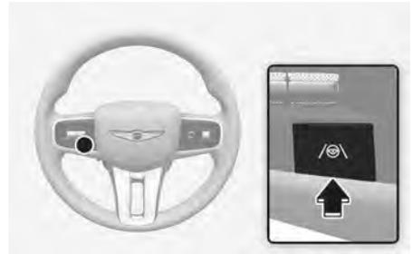
With the engine on, press the Lane Driving Assist (/Ⓢ) button located on the steering wheel to turn on Lane Following Assist. The gray or green Ⓢ indicator light illuminates on the instrument cluster.
