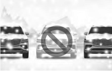
Snow may interfere with sensor operation, or Remote Smart Parking Assist may cancel if the road is slippery where you are parking.
