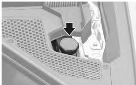
Check the fluid level in the reservoir periodically. The fluid level must be between the **MAX** (Maximum) and **MIN** (Minimum) marks on the side of the reservoir.
