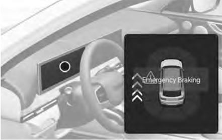
To warn you of a potential collision, the warning light on side view mirror and head-up display (if equipped) may blink, a warning message may appear on the instrument cluster, an audible warning may sound, and the steering wheel may vibrate.
