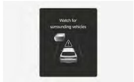
The "**Watch for surrounding vehicles**" warning message appears on the instrument cluster, and an audible warning sounds if the vehicle in front disappears when Smart Cruise Control is maintaining the distance from the vehicle ahead while driving below a certain speed.
