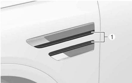
If the LED light (1) does not operate, contact an authorized retailer of Genesis Branded products.
