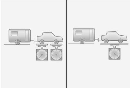
The tongue load is an important weight to measure because it affects the total Gross Vehicle Weight (GVW) of your vehicle. The trailer tongue should weigh a minimum of 10 % of the total loaded trailer weight, within the limits of the maximum (15 %) trailer tongue load permissible.
