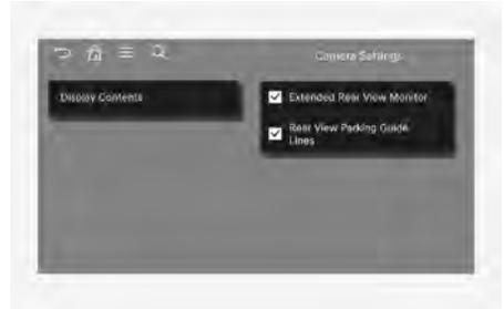
To change the settings of Rear View Monitor's display contents, press the setup icon (⚙️) on the screen while Rear View Monitor is operating, or select **Setup > Vehicle > Driver Assistance > Parking Safety > Camera Settings** from the Settings menu in the infotainment system while the engine is on.
