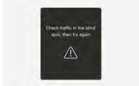
When Electric child safety lock is operating and an approaching vehicle from the rear area is detected, the rear doors cannot be unlocked even if you try to unlock the rear doors using the electronic child safety lock button. The warning light on the side view mirror may blink and the **"Check traffic in the blind spot, then try again"** warning message may appear on the instrument cluster.
