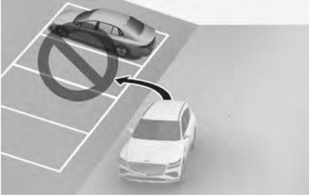
Remote Smart Parking Assist does not work normally on a inclined or curved road surface. Do not park even though the parking space is recognized by the sensor.
