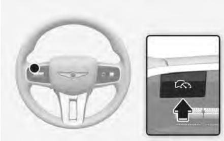
Press the Driving Assist (
