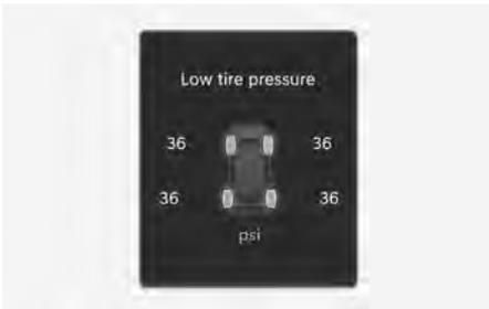
When the tire pressure monitoring system warning indicators are illuminated and a warning message displayed on the cluster display, one or more of your tires is significantly under-inflated. The Low Tire Pressure Position Telltale will indicate which tire is significantly underinflated by illuminating the corresponding parking light.
