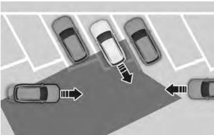
Rear Cross-Traffic Collision-Avoidance Assist may be limited when backing up diagonally, and may not detect any vehicle approaching from the left or right. If this occurs, the function may not activate a warning or brake your vehicle.
