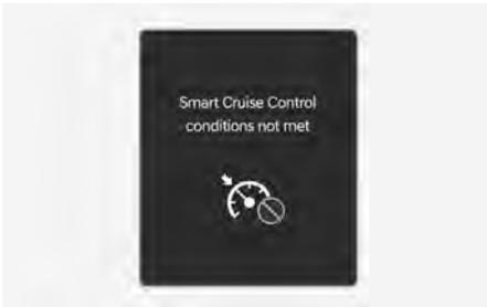
If the Driving Assist button, **+** switch, **-** switch or **||** switch is operated when Smart Cruise Control operating conditions are not satisfied, the "**Smart Cruise Control conditions not met**" or "**SCC (Smart Cruise Ctrl.) conditions not met**" message appears on the instrument cluster, and an audible warning sounds.
