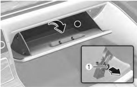
2. Remove the stoppers on both sides to allow the glove box to hang open.
