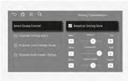
With the engine on, if **Setup > Vehicle > Driver Assistance > Driving Convenience > Smart Cruise Control > Based on Driving Style** is selected from the Settings menu, Smart Cruise Control operates based on your driving style, such as vehicle distance, acceleration, and reaction speed.
