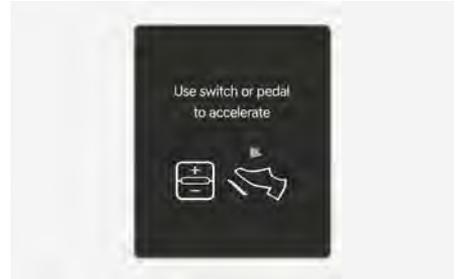
In traffic, your vehicle stops if the vehicle ahead of you stops. Also, if the vehicle ahead of you starts moving, your vehicle starts moving as well. In addition, after your vehicle has stopped and a certain time has passed, the "**Use switch or pedal to accelerate**" message appears on the instrument cluster. Depress the accelerator pedal or push the **+** switch, **-** switch, or **||** switch to start driving.
