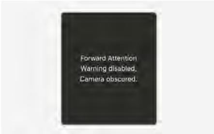
If there is an object right in front of the in-cabin camera or between you and the camera for a certain period of time Forward Attention Warning does not operate properly.
