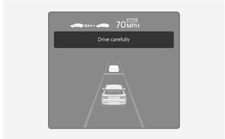
The "**Drive carefully**" warning message appears if Navigation-based Smart Cruise Control is not able to slow down your vehicle.
