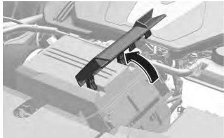
2. Pull down the lever to the UNLOCK position.
