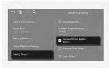
With the engine on, select **Setup** > **Vehicle** > **Driver Assistance** > **Driving Safety** > **Forward Cross-Traffic Safety** from the Settings menu to turn on Junction Crossing function and deselect to turn off the function.
