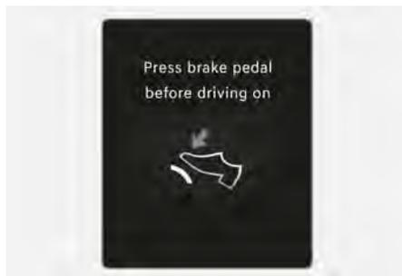
When the gear is shifted from N (Neutral) to R (Reverse), D (Drive) or Manual shift mode without the brake pedal depressed, a message will appear on the cluster display. To activate auto start, depress the brake pedal.
