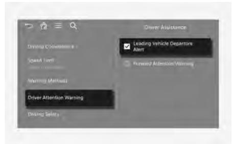
If **Leading Vehicle Departure Alert** is selected, the function informs you when a detected vehicle in front departs from a stop.
