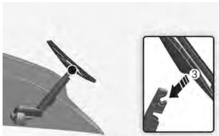
4. Rotate back the blade assembly so that it aligns with the wiper arm.
