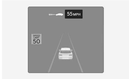
When driving at a speed higher than the displayed speed limit, the speed limit is blinking in red and the warning sounds.
