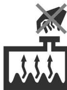
Never remove the engine coolant cap and/or liquid-cooled intercooler coolant cap or the drain plug while the engine and radiator are hot.
