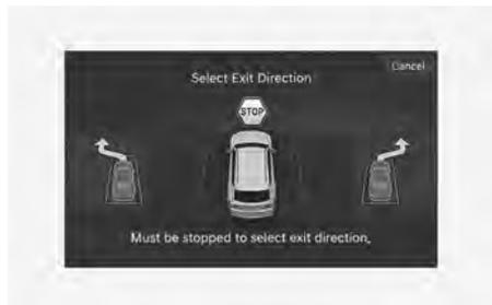
1. With the vehicle stopped by depressing the brake pedal, the infotainment system screen displays the possible directions for parallel exit.
