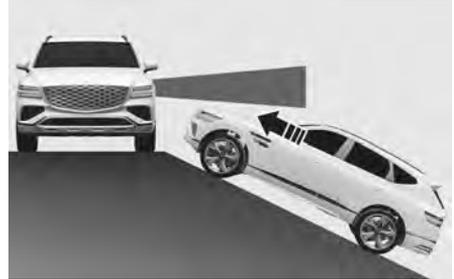
Rear Cross-Traffic Collision-Avoidance Assist may be limited when your vehicle is on an uphill or downhill slope, and may not detect any vehicle approaching from the left or right. If this occurs, the function may activate a warning and brake your vehicle even when not needed.
