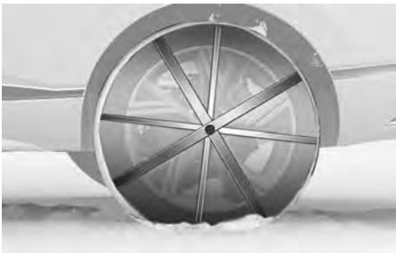
Since the sidewalls of radial tires are thinner than other types of tires, they may be damaged by mounting some types of tire chains on them. Therefore, the use of snow tires is recommended instead of tire chains. If tire chains must be used, use genuine Genesis parts and install the tire chain after reviewing the instructions provided with the tire chains. Damage to your vehicle caused by improper tire chain use is not covered by your vehicle manufacturer's warranty.
