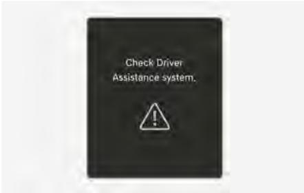
When Highway Driving Assist is not working properly, the "**Check Driver Assistance system.**" warning message may appear and the
