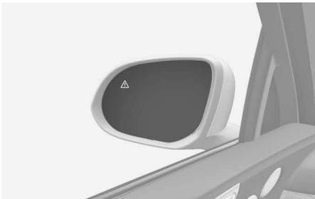
When a vehicle is detected in a blind spot, the warning light on the side view mirror and head-up display (if equipped) may illuminate.
