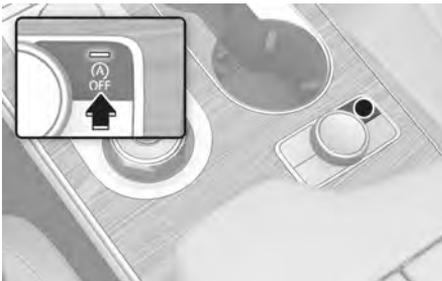
Press the ISG OFF (A) button to turn off the ISG system. The ISG OFF (A) button indicator illuminates. To use the system, press the ISG OFF (A) button again.
