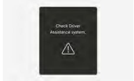
When Smart Cruise Control is not working properly, the "**Check Driver Assistance system.**" warning message may appear and the
