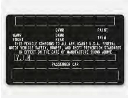
The certification label is located on the driver's door sill at the center pillar and shows the maximum allowable weight of the fully loaded vehicle. This is called the GVWR (Gross Vehicle Weight Rating). The GVWR includes the weight of the vehicle, all occupants, fuel and cargo. This label also tells you the maximum weight that can be supported by the front and rear axles, called Gross Axle Weight Rating (GAWR).
