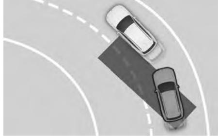
Blind-Spot Collision-Avoidance Assist may detect a vehicle in the same lane when driving on curves and activate a warning and brake your vehicle.
