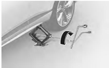
9. Loosen a wheel bolt with the wheel lug wrench and remove it with your fingers.
