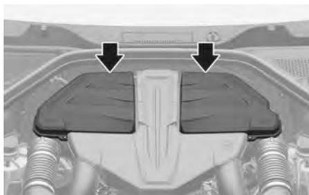
Do not attempt to wash or rinse it, because water can damage the filter. If soiled, the air cleaner filter must be replaced. Visit an authorized retailer of Genesis Branded products to replace air cleaner filter. Replace the air cleaner filter according to the Maintenance Schedule.
