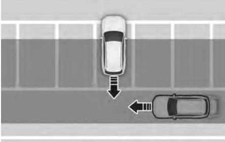
Rear Cross-Traffic Collision-Avoidance Assist may detect vehicles passing by behind you when parking in reverse into a parking space. If this occurs, the function may activate a warning and brake your vehicle even when not needed.
