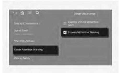
With the engine on, select **Setup > Vehicle > Driver Assistance > Driver Attention Warning** from the Settings menu in the infotainment system to select the following:
