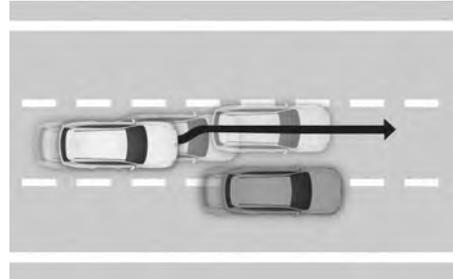
When vehicle speed is above 40 mph (60 km/h), if a detected vehicle around you is driving at a close distance, your vehicle controls the steering in the opposite direction of the vehicle. If a vehicle is detected at both sides of the lane and are driving close to you, the function does not veer to the opposite side of the lane.
