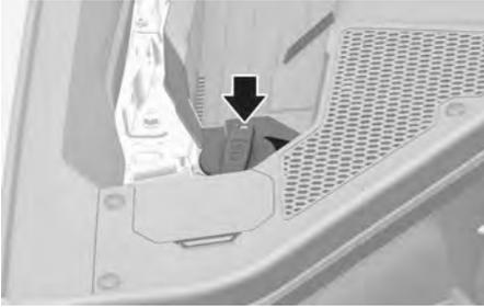
Check the fluid level in the washer fluid reservoir and add fluid if necessary. Plain water can be used if washer fluid is not available. However, use washer fluid with antifreeze in cold climates to prevent freezing.
