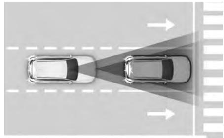
Forward Collision-Avoidance Assist helps detect a vehicle, a powered two-wheeler, a pedestrian, or a cyclist ahead on the road and may warn you of a possible collision with a warning message on the instrument cluster and a warning sound. Also, Forward Collision-Avoidance Assist may assist with braking your vehicle to help reduce collision speed or help avoid a collision.
