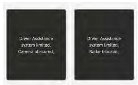
If the front view camera, front radar, bumper, or sensor is covered or blocked by foreign material, such as snow, rain, or dirt, or when a trailer or hitch mounted carrier is installed, the detecting performance may decrease and temporarily limit or disable Forward Collision-Avoidance Assist.
