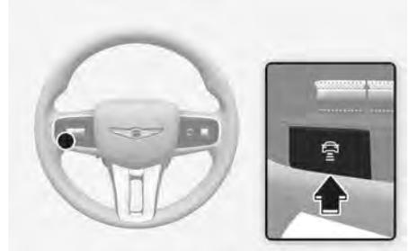
Each time the button is pressed, the vehicle distance changes as follows:
