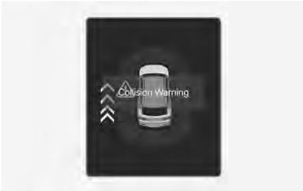
When an approaching vehicle from the rear is detected while a door is being opened, the warning light on the side view mirror may blink, the **"Collision Warning"** warning message may appear on the instrument cluster, and an audible warning may sound.
