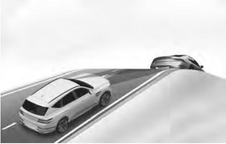
During uphill or downhill driving, Smart Cruise Control may not detect a moving vehicle in your lane, and cause your vehicle to accelerate to the set speed. Also, your vehicle speed rapidly decreases when a vehicle ahead is detected suddenly.
