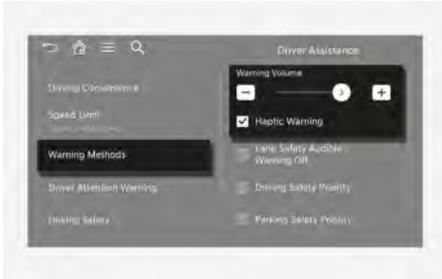
With the engine on, select **Setup > Vehicle > Driver Assistance > Warning Methods** from the Settings menu in the infotainment system to select the following:
