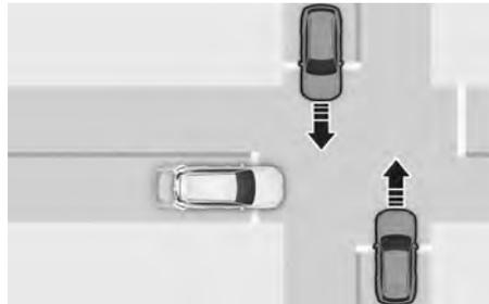
Junction Crossing function helps avoid a collision with oncoming vehicles on the left or right side when crossing an intersection by applying emergency braking.
