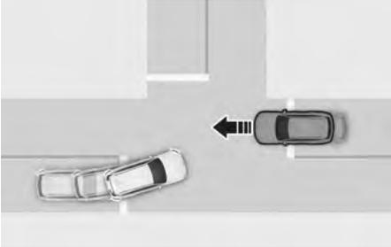
Junction Turning function helps avoid a collision with an oncoming vehicle or powered two-wheeler in an adjacent lane when turning left at a crossroad with the turn signal on by applying emergency braking.
