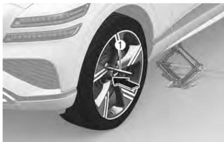
11. Remove the wheel from the studs and lay it flat on the ground out of the way. Remove any dirt or debris from the studs, mounting surfaces, and spare tire.
