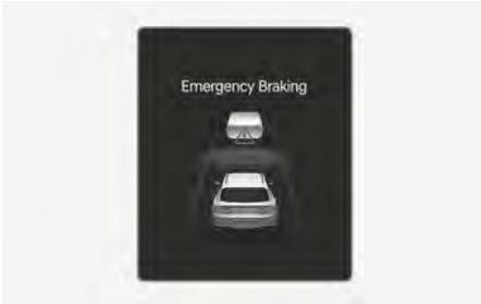
To warn the driver that emergency braking is assisted, the
