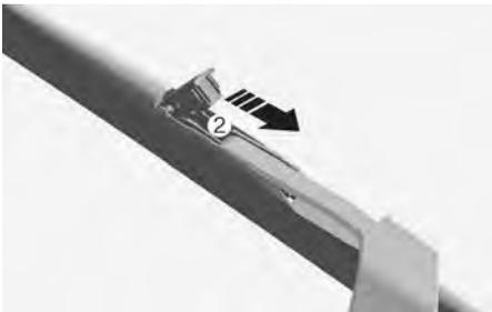
5. Remove the wiper blade from the wiper arm.
