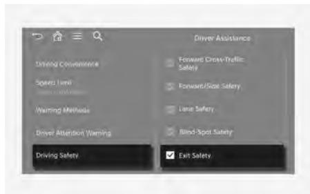
With the engine on, select **Setup > Vehicle > Driver Assistance > Driving Safety > Exit Safety** from the Settings menu in the infotainment system to turn on Safe Exit Assist and deselect to turn off the function.
