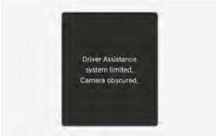
If the front view camera is covered or blocked, its detecting performance is reduced, and Intelligent Speed Limit Assist is temporarily limited or disabled.
