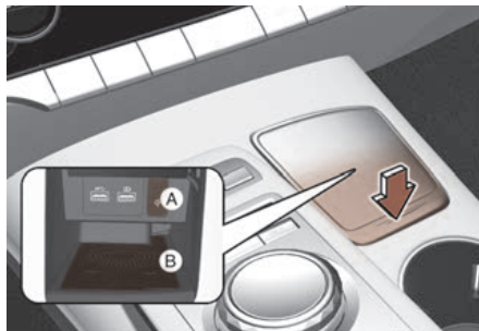
[A] Indicator light [B] Charging pad
