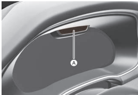
[A] Interior view camera
