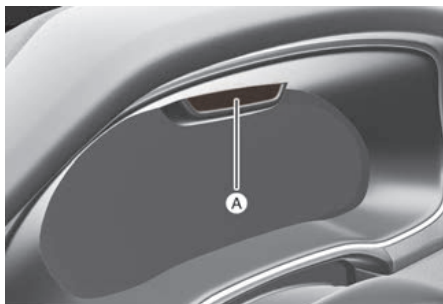
[A] Interior view camera
