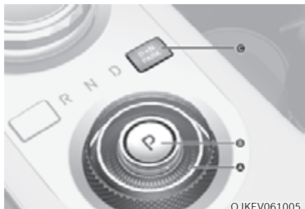
[A]: Rotary shifter, [B]: P button, [C]: P>N PARK button
