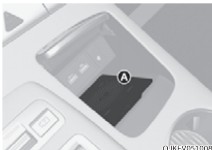
[A]: In-vehicle authentication pad (Wireless charging pad)
