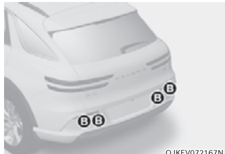
[B]: Rear ultrasonic sensor
