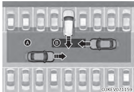
[A]: Rear Cross-Traffic Collision Warning operating range,
