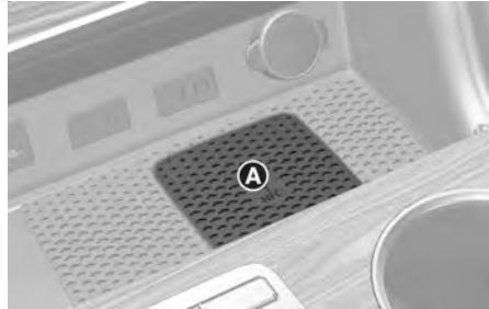
[A] Vehicle authentication pad (Wireless charging pad)
