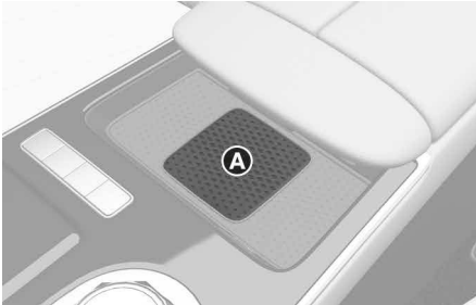
[A] Vehicle authentication pad (wireless charging pad)
