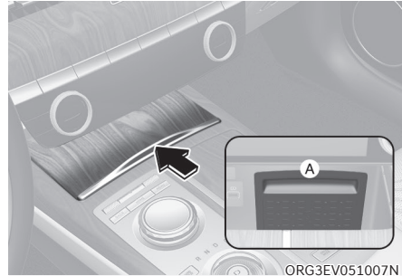
[A] : In-vehicle authentication pad (Wireless charging pad)
