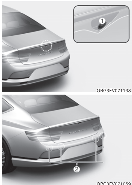
[1] : Rear view camera, [2] : Rear ultrasonic sensors
