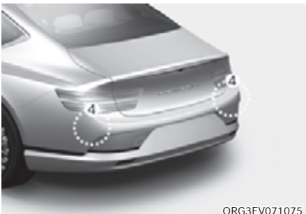
[1]: Front view camera, [2]: Front radar, [3]: Front corner radar (if equipped), [4]: Rear corner radar
