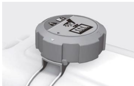
Liquid-cooled intercooler coolant
