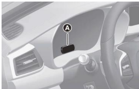
[A] Interior view camera
