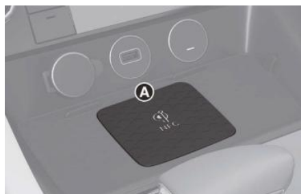
[A] Vehicle authentication pad (Wireless charging pad)
