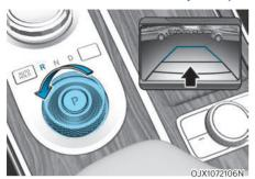
Rear View Monitor displays the area behind your vehicle to help with safe parking.
