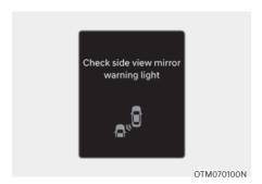
When the side view mirror warning light is not working properly, the 'Check side view mirror warning light' warning message will appear on the cluster for several seconds, and the master (A) warning light will illuminate on the cluster. If this occurs, have the vehicle inspected by an authorized retailer of Genesis Branded products.
