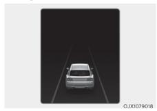
The status of Smart Cruise Control, Lane Following Assist, Highway Driving Assist, etc., is displayed when Driving Assist view is selected.
