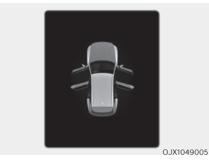
This warning is displayed if any door or hood or liftgate is left open. The warning will indicate which door are open in the display.
