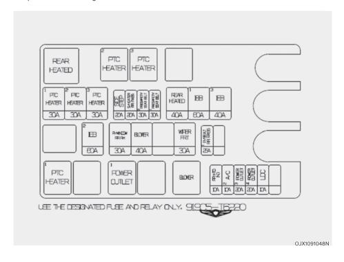
Engine compartment fuse panel (Engine room sub junction block)
