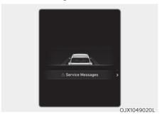
When Service Messages menu is selected, press the OK switch on the steering wheel to check vehicle warning messages.
