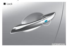
Touch the touch sensor on the front outside door handle (the engraved part) while carrying the Smart Key with you or press the Door Lock button on the Smart Key, all doors will lock.
