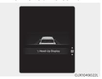
When Head-Up Display menu is selected, press the OK switch on the steering wheel. You can select or deselect head-up display by pressing the OK switch.
