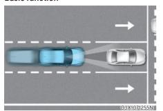
Forward Collision-Avoidance Assist detects a vehicle, a powered-two wheeler, a pedestrian, or a cyclist ahead on the road and may warn you of a possible collision with a warning message on the instrument cluster and a warning sound. Also, Forward Collision-Avoidance Assist may assist with braking your vehicle to help reduce collision speed or avoid a collision.
