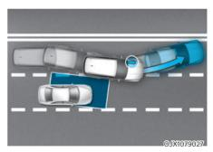
When changing lanes by detecting the lane ahead, if Blind-Spot Collision-Avoidance Assist detects that there is a collision risk with an approaching vehicle in the blind spot, It can help avoid a collision by applying the brake.
