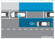
While your vehicle is stopped, and if Safe Exit Assist detects a vehicle approaching the rear corner of your vehicle and a passenger opens a door, Safe Exit Assist may warn you with a warning message and a warning sound to help avoid a collision.
