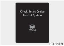
When Smart Cruise Control is not working properly, the 'Check Smart Cruise Control system' warning message will appear, and the /\ warning light will illuminate on the cluster. Have the vehicle inspected by an authorized retailer of Genesis Branded products.
