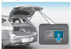
Press the power liftgate lock button while carrying the smart key. The liftgate closes and locks with a warning sound. Additionally, all doors will lock.
