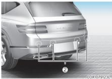
[1]: Rear view camera, [2]: Rear ultrasonic sensors
