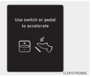
In traffic, your vehicle will stop if the vehicle ahead of you stops. Also, if the vehicle ahead of you starts moving, your vehicle will start as well. In addition, after the vehicle has stopped and a certain time have passed, the 'Use switch or pedal to accelerate' message will appear on the cluster. Depress the accelerator pedal or operate the + switch, - switch or II' switch to start driving.
