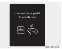
When Highway Driving Assist is operating, your vehicle will stop if the vehicle ahead of you stops. Also, if the vehicle ahead of you starts moving within 30 seconds after the stop, your vehicle will start as well. In addition, after the vehicle has stopped and 30 seconds have passed, the 'Use switch or pedal to accelerate' message will appear on the cluster. Depress the accelerator pedal or push the + switch, - switch or II S switch to start driving.
