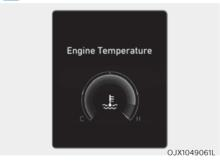
For 8-inch instrument cluster, you can check the engine coolant temperature in the Utility view on the cluster.
