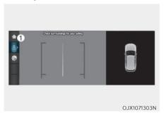
When you touch the icon (1), the top view is displayed on the screen and shows the distance from the vehicle in the back of your vehicle while parking.
