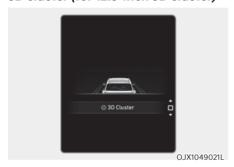
When 3D Cluster menu is selected, press the OK switch on the steering wheel. You may select or deselect 3D cluster effect by pressing the OK switch.
