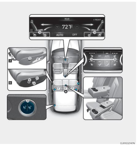
[A]: Manual adjustment, [B]: Power adjustment (5-seater)
