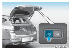
Press the power liftgate open/close button. The liftgate opens or closes with a warning sound.
