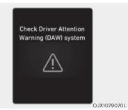
When Driver Attention Warning is not working properly, the 'Check Driver Attention Warning (DAW) system' warning message will appear on the cluster for several seconds, and the master \( \tilde{\Lambda} \) warning light will illuminate on the cluster. If this occurs, have the vehicle inspected by an authorized retailer of Genesis Branded Products.
