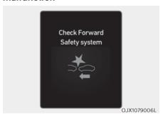
When Forward Collision-Avoidance Assist is not working properly, the 'Check Forward Safety system' warning message will appear, and the 🛬 and 🛆 warning lights will illuminate on the cluster. Have the vehicle inspected by an authorized retailer of Genesis Branded products.
