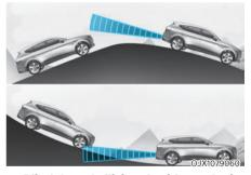
Blind-Spot Collision-Avoidance Assist may not operate properly when driving on a slope. The function may not detect the vehicle in the next lane or may incorrectly detect the ground or structure.
