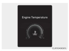
Engine temperature (for 8-inch cluster) Engine coolant temperature gauge display shows the temperature of the engine coolant when the engine is running.
