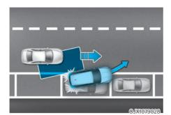
When you are driving forward out of a parking space, if Blind-Spot Collision-Avoidance Assist judges that there is a collision risk with an approaching vehicle in the blind spot, Blind-Spot Collision-Avoidance Assist will help avoid a collision by applying the brake.
