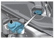
Check the fluid level in the reservoir periodically. The fluid level should be between MAX and MIN marks on the side of the reservoir
