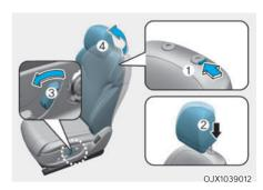
To reinstall the head restraint:
