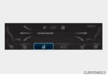
While the engine is running, touch the heated steering wheel icon to warm the steering wheel.
