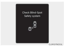
When Blind-Spot Collision-Avoidance Assist is not working properly, the 'Check Blind-Spot Safety system' warning message will appear on the cluster for several seconds, and the master A warning light will illuminate on the cluster. If this occurs, have the vehicle inspected by an authorized retailer of Genesis Branded products.
