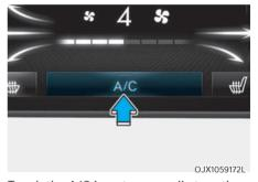
Touch the A/C icon to manually turn the air conditioning on (indicator light ON) and off.
