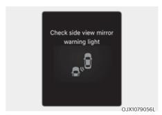
When the side view mirror warning light is not working properly, the 'Check side view mirror warning light' warning message will appear on the cluster for several seconds, and the master warning light will illuminate on the cluster. If this occurs, have the vehicle inspected by an authorized retailer of Genesis Branded products.
