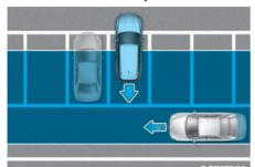
Rear Cross-Traffic Collision-Avoidance Assist may detect vehicles passing by behind you when parking in reverse into a parking space.
