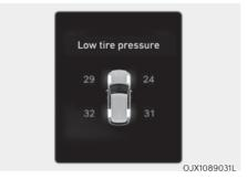
When the tire pressure monitoring system warning indicators are illuminated and a warning message displayed on the cluster display, one or more of your tires is significantly under-inflated. The Low Tire Pressure Position Telltale will indicate which tire is significantly underinflated by illuminating the corresponding position light.
