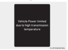
This message is displayed when the transmission oil temperature is high.
