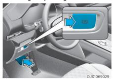
To release EPB (Electronic Parking Brake):
