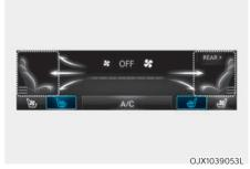
While the engine is running, touch either of the seat warmer icons to warm the driver's seat or front passenger's seat.  Manual temperature control Each time you touch the icon, the temperature setting of the seat is changed as follows:
