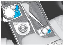
Press the AUTO LOCK button to change from Auto AWD (ﷺ indicator light off) mode to AWD Lock mode (ﷺ indicator light on).
