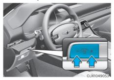
When the vehicle's position lights or headlights are on, press the illumination control switch to adjust the brightness of the instrument panel illumination.
