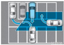
Rear Cross-Traffic Collision-Avoidance Assist may detect vehicles which are parking or pulling out near your vehicle (for example, a vehicle leaving beside your vehicle, a vehicle parking or pulling out in the rear area, a vehicle approaching your vehicle making a turn, etc.). If this occurs, the function may unnecessarily warn the driver and control the brake.
