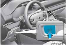
Press the power liftgate open/close button for 1 second. The liftgate opens or closes with a warning sound.
