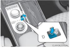
4. Remove the cap-cover (1) and press the button (2) while depressing the brake pedal.
