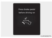
Press brake pedal before driving on When the gear is shifted from N (Neutral) to R (Reverse), D (Drive) or Manual shift mode without the brake pedal depressed, a message will appear on the cluster display. To activate auto start, depress the brake pedal.
