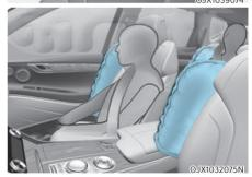
Your vehicle is equipped with a side air bag in each front and outboard second row seat. Additionally, a front center side air bag is provided in the inboard side of the driver seatback. The purpose of the air bag is to provide the vehicle's additional protection than that offered by the seat belt alone.
