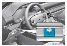
When the system is deactivated, the ISG off button indicator will illuminate and a message 'Auto Stop error. Shift to P or N to start engine manually' appears on the cluster display with a warning sound.
