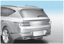
[1]: Front view camera, [2]: Rear corner radar Refer to the picture above for the detailed location of the detecting sensors.
