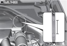
Pull the dipstick out again and check the level. The level should be between F (Full) and L (Low).
