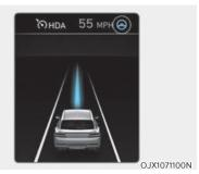
If the vehicle ahead and/or both lane markings are detected and your vehicle speed is below 120 mph (200 km/h), the green indicator light will illuminate on the cluster, and Lane Following Assist will help center the vehicle in the lane by assisting the steering wheel.
