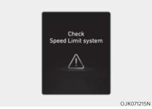
When Intelligent Speed Limit Assist is not working properly, the 'Check Speed Limit system' warning message will appear on the cluster for several seconds, and the master (/\h) warning light will illuminate on the cluster. If this occurs, have the vehicle inspected by an authorized retailer of Genesis Branded products.
