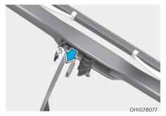
5. Remove the wiper blade from the wiper arm (5).
