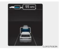
If you want to speed up temporarily when Smart Cruise Control is operating, depress the accelerator pedal. While the speed is increasing, the set speed, distance level and target distance will blink on the cluster.
