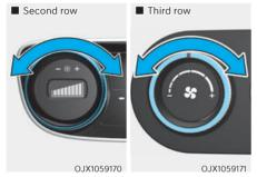
The fan speed can be set to the desired speed by touching the \$\mathbb{s}\$ or \$\mathbb{s}\$ icon, or by turning the fan speed control knob.
