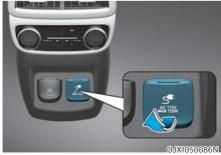
The AC inverter supplies 115 volts (150 watts) electric power to operate electric accessories or equipment.
