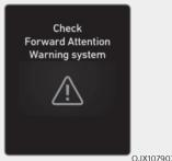
When Forward Attention Warning is not working properly, the 'Check Forward Attention Warning system' warning message will appear on the cluster. If this occurs, have the vehicle inspected by an authorized retailer of Genesis Branded products.
