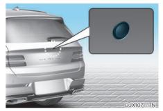
The wide-rear view camera is used as a detecting sensor to detect pedestrians. If the camera lens is covered with foreign material, such as snow or rain, it may adversely affect camera performance and Reverse Parking Collision-Avoidance Assist may not operate normally. Always keep the camera lens clean.
