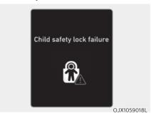
When electronic child safety lock does not work even though the button is pressed, the message will be displayed and an alarm will sound. If this occurs, have the vehicle inspected by an authorized retailer Genesis Branded products.
