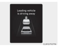
When the front vehicle departs from a stop, Leading Vehicle Departure Alert will inform the driver by displaying the 'Leading vehicle is driving away' message on the cluster and an audible warning will sound.
