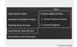
Select 'Ergo-Motion Seat' from the infotainment system's Settings menu to select and set up supplemental functions.
