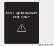
When High Beam Assist is not working properly, the 'Check High Beam Assist (HBA) system' warning message will appear and /\(\Lambda\) warning light will illuminate on the cluster display. Have the function inspected by an authorized retailer of Genesis Branded products.
