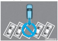
Remote Smart Parking Assist does not provide diagonal parking. Even if your vehicle was able to enter the parking space, do not use the function because the function cannot operate normally.
