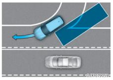
Blind-Spot Collision-Avoidance Assist may not operate properly when driving where the road merges or divides. The function may not detect the vehicle in the next lane. Always pay attention to road and
