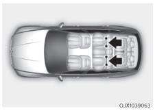
LATCH anchors have been provided in the left and right outboard rear seating positions. Their locations are shown in the illustration.
