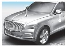
[1], [2] : Wide-side view camera (camera located at bottom of the mirror)
