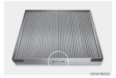
Install a new cabin air filter in the correct direction with the arrow symbol (↓) facing downwards, to prevent noise and reduce effectiveness.
