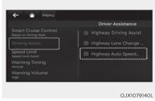
With the engine on, select 'Driver Assistance → Driving Assist → Highway Auto Speed Change' from the Settings menu to turn on Navigation-based Smart Cruise Control and deselect to turn off the function.
