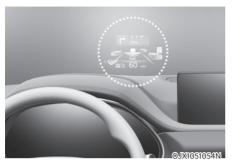
The Head-Up Display is a feature that allows the driver to view information projected onto a transparent screen while still keeping their eyes on the road ahead while driving.
