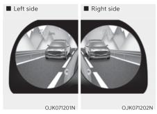
Blind-Spot View Monitor uses the wideside view cameras to display the rear blind spot areas of your vehicle on the instrument cluster when the turn signal is turned on to help with safe lane changes.
