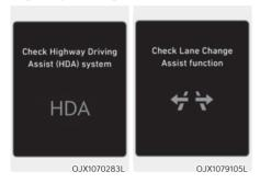
When Highway Driving Assist or Highway Lane Change function is not working properly, the 'Check Highway Driving Assist (HDA) system' or 'Check Lane Change Assist function' warning message will appear, and the \( \underset \) warning light will illuminate on the cluster. Have the vehicle inspected by an authorized retailer of Genesis Branded products.
