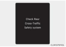
When Rear Cross-Traffic Collision-Avoidance Assist is not working properly, the 'Check Rear Cross-Traffic Safety system' warning message will appear on the cluster for several seconds, and the master warning light will illuminate on the cluster. If this occurs, have the vehicle inspected by an authorized retailer of Genesis Branded products.
