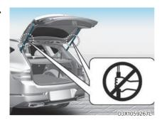
Do not grab or hold on to the liftgate support struts at any time. Damage to the liftgate support struts could result. Deformation of the liftgate support struts may cause vehicle damage and personal injury may occur.
