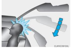
Be careful when closing the liftgate with passenger's seated on the third row seat. If the passenger's head is not properly against an adjusted head restraint or a tall person is seated, the liftgate may hit the passenger's head, which could cause injury.
