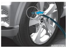
4. Unscrew the valve cap from the valve of the defective and screw the filling hose (3) of the sealant bottle onto the valve
