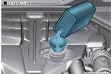
7. If the oil level is near or below L, add enough oil to bring the level to F.
