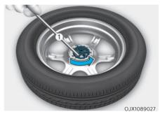
If it is hard to loosen the tire hold-down wing bolt by hand, you can loosen it easily using the wheel lug wrench (1). Turn the tire hold-down wing bolt counterclockwise with the wheel lug wrench.
