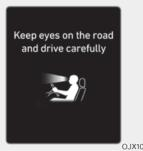
Forward Attention Warning determines whether the driver is focused on the road depending on information, such as the amount of time the driver is looking elsewhere, the amount of time the eyes are closed, how frequently the driver yawns, etc. If Forward Attention Warning judges the driver is not focused, the 'Keep eyes on the road and drive careful' warning message will appear on the cluster, and an audible warning will sound.
