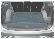
To keep items from shifting in the cargo area, you can use the 4 holders located in the luggage board to attach a cargo net.
