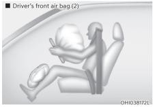
Upon deployment, tear seams molded directly into the pad covers will separate under pressure from the expansion of the air bags. Further opening of the covers allows full inflation of the air bags.
