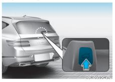
When the liftgate is closed, press the power liftgate open/close button to open the liftgate.
