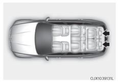
The third row seats are equipped with head restraints in all the seating positions for the passenger's safety and comfort.
