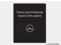
When Lane Following Assist is not working properly, the 'Check Lane Following Assist (LFA) system' warning message will appear on the cluster for several seconds, and the master \( \triangle \) warning light will illuminate on the cluster. If this occurs, have the vehicle inspected by an authorized retailer of Genesis Branded products.
