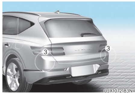
[1] : Front view camera, [2] : Front radar, [3] : Rear corner radar
