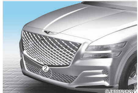
[1] : Front view camera, [2] : Front radar
