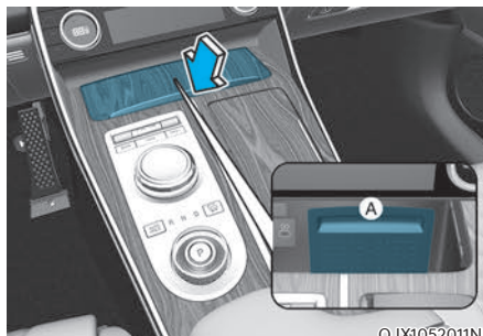
[A] : In-vehicle authentication pad (Wireless charging pad)
