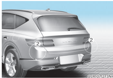
[1] : Front view camera, [2] : Rear corner radar
