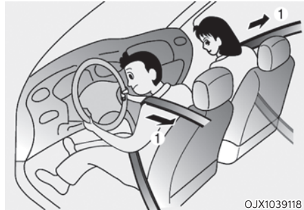
[1] : Retractor pre-tensioner seat belt (Driver and front passenger)
