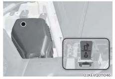
Pull the yellow label in the high voltage cut-off switch to shut down the high voltage battery.
