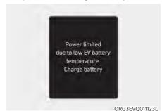
Both warning messages are displayed to protect electric vehicle system when outside temperature is low. If the high voltage battery charging level is low and parked outside in low temperature for a long time, vehicle power may be limited. Charging the battery before driving helps
