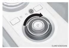
To shift the gear to D (Drive), rotate the rotary shifter to D (Drive) while depressing the brake pedal.
