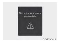
When the side view mirror warning light is not working properly, the 'Check side view mirror warning light' warning message will appear on the instrument cluster for several seconds, and the master (/\) warning light will illuminate on the instrument cluster. If this occurs, have the vehicle inspected by an authorized retailer of Genesis Branded products.
