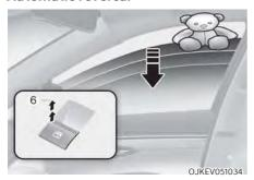
If a window senses any obstacle while it is closing automatically, it will stop and lower about 12 inches (30 cm) to allow the object to be cleared.
