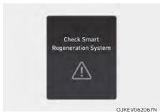
When the front radar is covered or blocked, the smart regeneration system may be temporarily disabled.
