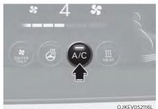
Press the A/C icon to manually turn the air conditioning on (indicator light ON) and off.
