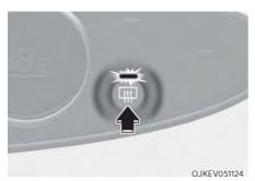
The defroster heats the window to remove frost, fog and thin ice from the interior and exterior of the rear window, while the vehicle is on (READY indicator on).
