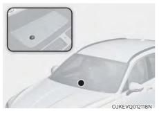
The high voltage indicator is located on top of the dashboard. When the 12 V auxiliary battery is discharged, it is charged from the high voltage battery of the vehicle. When the high voltage electricity flows in the vehicle, the color of the indicator changes to amber and turns off after charging is finished.
