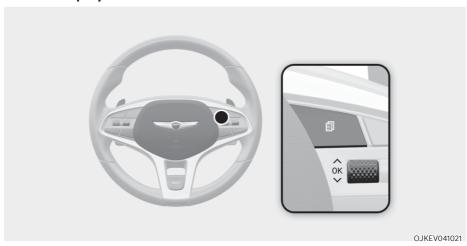
The cluster display modes can be changed by using the control switches.
