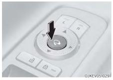
Press the button to fold or unfold the side view mirrors.
