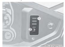
When scheduled charging is set and the AC charger or the portable charger (ICCB: In-Cable Control Box) is connected for charging, the indicator lamp illuminates (1) for 3 minutes to indicate that scheduled charging is set.
