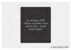
To release EPB, fasten seatbelt and close door, hood and liftgate
