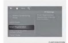
To adjust the regenerative braking level of the smart regeneration system, go to 'Setup > EV > Smart Regeneration' from the infotainment system.
