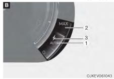
The instrument cluster displays 'AUTO' (1) when the smart regeneration system is on. Depending on the conditions, the system adjusts the regenerative braking level (2). The indicator light (3) illuminates when the vehicle recognizes a vehicle.
