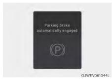
Parking brake automatically engaged When EPB is applied while Auto Hold is activated, a warning will sound and a message will appear.
