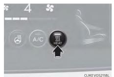
Press the HEAT icon to turn the heater on (indicator light will illuminate).
