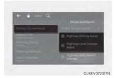
With the vehicle on, select or deselect **Setup > Vehicle > Driver Assistance > Driving Convenience** from the Settings menu to set whether to use each function.
