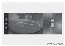
The rear image is displayed on the screen when the gear is in P (Park) to assist in parking. Using the view button (2) you may select top view, rear view and side view.
