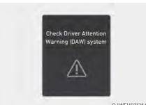
When Driver Attention Warning is not working properly, the 'Check Inattentive Driving Warning system' warning message will appear on the instrument cluster for several seconds, and the master (\hat{\Lambda}) warning light will illuminate on the instrument cluster. If this occurs, have the vehicle inspected by an authorized retailer of Genesis Branded products.
