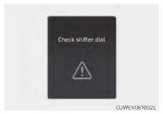
This message is displayed when there is a malfunction with the rotary shifter.
