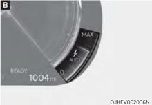
The smart regeneration system turns on and the regenerative braking level is displayed as 'AUTO'.
