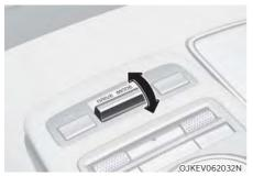
The mode changes, as the following, whenever the DRIVE MODE switch is pushed up or down.
