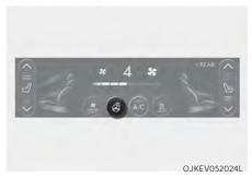
While the vehicle is on (**READY** indicator on) touch the heated steering wheel icon to warm the steering wheel.
