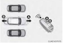
(1) Press and hold one of the Forward (()) or Backward (()) button on the smart key. Remote Smart Parking Assist will automatically control the steering wheel, vehicle speed and gearshift. The vehicle will move in the direction of the button pressed.
