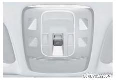
The sunroof can only be operated when the Start/Stop button is in the ON or START position.
