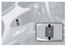
When the vehicle's parking lights or headlight are on, press the illumination control switch to adjust the brightness of the instrument panel illumination.
