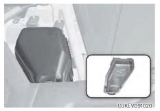
Inside the fuse panel cover, you can find the fuse label describing fuse names and ratings.
