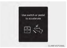
When Highway Driving Assist is operating, your vehicle will stop if the vehicle ahead of you stops. Also, if the vehicle ahead of you starts moving within 30 seconds after the stop, your vehicle will start as well. In addition, after the vehicle has stopped and 30 seconds have passed, the 'Use switch or pedal to accelerate' message will appear on the cluster. Depress the accelerator pedal or operate the + switch, - switch or II'D switch to start driving.
