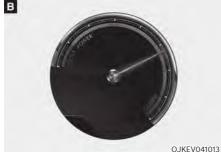
The Power/Charge gauge shows the energy consumption and recovery status of the electric motor.
