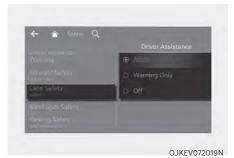
With the vehicle on, select or deselect Setup > Vehicle > Driver Assistance > Lane Safety from the Settings menu to set whether to use each function.
