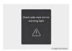
When the side view mirror warning light is not working properly, the 'Check side view mirror warning light' warning message will appear on the instrument cluster for several seconds, and the master (A) warning light will illuminate on the instrument cluster. If this occurs, have the vehicle inspected by an authorized retailer of Genesis Branded products.
