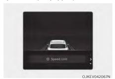
When the Speed Unit menu is selected, press the **OK** button on the steering wheel. You can change the speed unit setting between MPH and km/h for the
