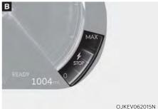
The selected regenerative braking level appears on the instrument cluster.
