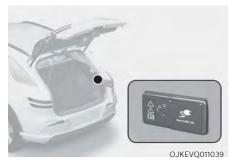
V2L(Vehicle to Load) is installed on the lower right side of the cargo area. V2L is a convenient feature which provides electricity to use diverse household electrical appliances in the vehicle.
