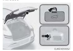
To unlock and open the liftgate manually from inside the cargo area, perform the following procedure:
