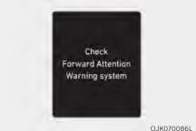
When Forward Attention Warning is not working properly, the 'Check Forward Attention Warning system' warning message will appear on the instrument cluster. If this occurs, have the vehicle inspected by an authorized retailer of Genesis Branded products.
