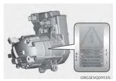
A compressor label informs you the type of compressor your vehicle is equipped with such as model (1), serial number (2), supplier part number (3), lot number (4), refrigerant oil (5) and refrigerant (6).
