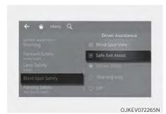
With the vehicle on, select Setup > Vehicle > Driver Assistance > Blind-Spot Safety > Safe Exit Assist from the Settings menu to turn on Safe Exit Assist and deselect to turn off the function.
