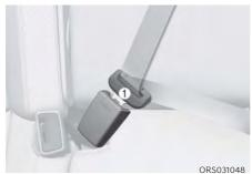
Insert the tongue plate (1) into the buckle until an audible "click" is heard, indicating the latch is locked. Pull the shoulder portion of the belt to snug the belt across your hips and remove slack.
