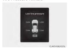
When the tire pressure monitoring system warning indicators are illuminated and a warning message displayed on the cluster display, one or more of your tires is significantly under-inflated. The Low Tire Pressure Position Telltale will indicate which tire is significantly underinflated by illuminating the corresponding position light.
