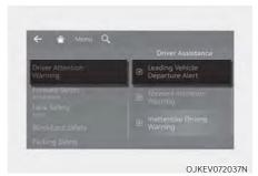
If Leading Vehicle Departure Alert is selected, the function will inform the driver when a detected vehicle in front departs from a stop.
