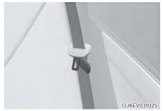
Route the seat belt webbing through the rear seat belt guides to prevent the belts from being trapped behind or under the seats.
