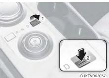
3. Remove the cap-cover (1) and press the button (2) while depressing the brake pedal.
