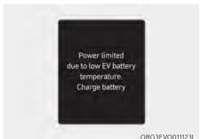
Both warning messages are displayed to protect electric vehicle system when outside temperature is low. If the high voltage battery charging level is low and parked outside in low temperature for a long time, vehicle power may be limited. Charging the battery before driving helps increase power.
