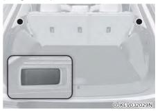
Pull the remote seatback release handle located on either side in the rear cargo area.
