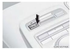
Press and hold the Parking Safety ( $P^m_{\underline{A}}$ ) button more than 2 seconds, to turn the Parking Collision-Avoidance Assist on or off.
