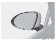
Your vehicle is equipped with both lefthand and right-hand side view mirrors. The mirrors can be adjusted remotely with mirror adjustment control switch. Adjust the side view mirrors to your desired position before driving.
