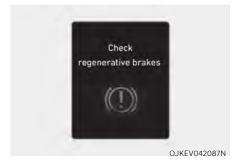
These warning messages are displayed when the regenerative brake system does not work properly.
