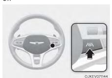
With the vehicle on, short press the Lane Driving Assist button located on the steering wheel to turn on Lane Following Assist. The grey or green (a) indicator light will illuminate on the cluster.
