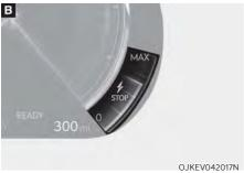
The selected regenerative braking level is displayed on the instrument cluster. Also, the Smart Regenerative System's operation status is displayed.
