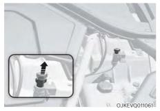
If the charging connector does not disconnect from the charging inlet due to battery discharge and failure of electric wires, open the hood and slightly pull the emergency cable. The charging connector is disconnected from the charging inlet.
