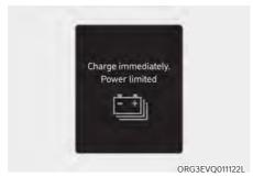
When the high voltage battery level reaches below about 5 %, this warning message is displayed.
