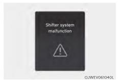
This message is displayed when the shift gear does not properly operate in the P (Park) position.
