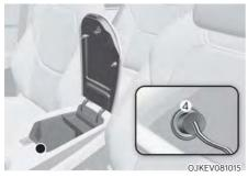
7. Plug the compressor power cord (4) into the vehicle power outlet.
