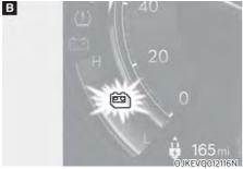
When the remaining battery is lower than 10 % on the SOC gauge, the High Voltage Battery Level ( warning light illuminates to alert you of the battery level.
