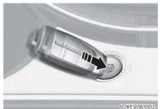
If the smart key battery is weak or the smart key does not work correctly, press the Start/Stop button with the smart key in the direction of the picture shown above.
