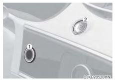
Place your finger on the fingerprint sensor (1) to verify your fingerprint. After it is successfully verified, start the vehicle by pressing the Start/Stop button (2) within 30 seconds.
