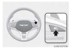
Press the Driving Assist button to turn Smart Cruise Control off.
