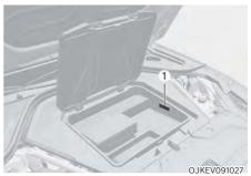
If the LED light (1) does not operate, contact an authorized retailer of Genesis Branded products for replacement.
