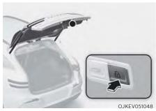
Press the power liftgate lock button while carrying the smart key. The liftgate closes and locks automatically. Additionally, all doors will lock. The liftgate can be closed and locked, and all doors locked only when the button is pressed while the vehicle is turned off (READY indicator off).
