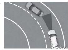
The front sensor may not detect the vehicle ahead if you are coasting on a curve. The regenerative braking intensity may automatically decrease and accelerate the vehicle.
