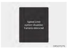
When the front windshield where the front view camera is located is covered with foreign material, such as snow or rain, it can reduce the detecting performance and temporarily limit or disable Intelligent Speed Limit Assist. If this occurs, the 'Speed Limit system disabled. Camera obscured' warning message will appear on the instrument cluster.
