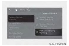
With the vehicle on, select or deselect **Setup > Vehicle > Driver Assistance** > **Driver Attention Warning** from the Settings menu to set whether to use each function.
