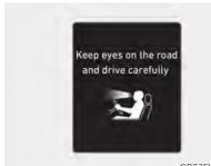
Forward Attention Warning determines whether the driver is focused on the road depending on information, such as the amount of time the driver is looking elsewhere, the amount of time the eyes are closed, how frequently the driver yawns, etc. If Forward Attention Warning judges the driver is not focused. the 'Keep eyes on the road and drive careful' warning message will appear on the cluster, and an audible warning will sound.
