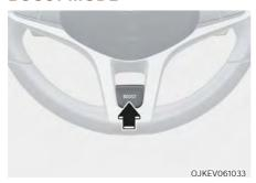
Boost mode maximizes motor performance for about 10 seconds for rapid acceleration.
