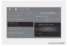
With the vehicle on, select or deselect **Setup > Vehicle > Driver Assistance > Speed Limit** from the Settings menu to set whether to use each function.
