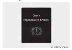
This warning message is displayed when the regenerative brake system does not work properly. In this case, have the vehicle inspected by an authorized retailer of Genesis Branded products.
