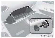
(2) Remove the stoppers on both sides to allow the glove box to hang open.
