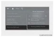
With the vehicle on, go to **Setup > Vehicle > Driver Assistance > Warning Methods** from the Settings in the infotainment system to select the following:
