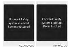
When the front view camera or radar is blocked or obscured by foreign material, rain, or snow, it can reduce the detecting performance and temporarily limit or disable Forward Collision-Avoidance Assist.
