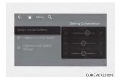
With the vehicle on, select Setup > Vehicle > Driver Assistance > Driving Convenience > Smart Cruise Control from the setting menu, to change Distance, Acceleration, Reaction Speed manually.
