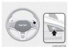
Press the Driving Assist (\*\*) button to turn Manual Speed Limit Assist off. The Speed Limit (\*\*) indicator will go off.
