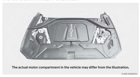
(1) Coolant reservoir ......9-12 (2) Brake fluid reservoir.....9-14 (3) Windshield washer fluid reservoir ...... 9-15 (4) Fuse box ...... 9-37
