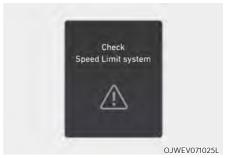
When Intelligent Speed Limit Assist is not working properly, the 'Check Speed Limit system' warning message will appear on the instrument cluster for several seconds, and the master (A) warning light will illuminate on the instrument cluster. If this occurs, have the vehicle inspected by an authorized retailer of Genesis Branded products.
