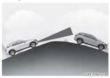
When coasting uphill or downhill, the front sensor may not detect the vehicle ahead or suddenly detect the vehicle ahead at the end of the incline or at the point where the incline changes. The regenerative braking intensity is adjusted automatically changing your vehicle speed. Brake as needed to reduce your driving speed.
