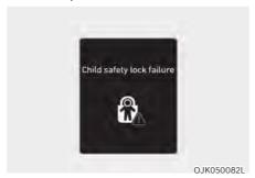
When electronic child safety lock does not work even though the button is pressed, the message will be displayed and an alarm will sound. Have the vehicle inspected by an authorized retailer Genesis Branded products.
