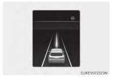
If the vehicle ahead and/or both lane markings are detected and your vehicle speed is below 120 mph (200 km/h), the green (A) indicator light illuminates on the cluster, and Lane Following Assist helps center the vehicle in the lane by assisting the steering wheel.
