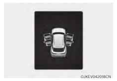
This warning is displayed if any door or hood or liftgate is left open. The warning indicates which door is open on the cluster display
