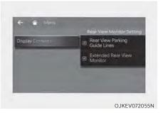
You can change Rear View Monitor Display Contents by touching the setup icon (②) on the screen while Rear View Monitor is operating, or selecting Driver Assistance > Parking Safety > Camera Settings from the Settings menu while the vehicle is on.
