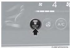
If you press the DRIVER ONLY icon (\$\mathbb{G}^{\text{RIVER}}\_{\text{ONLY}}\$) and the indicator light illuminates in the infotainment climate control screen, cold air mostly blows towards the driver's seat. However, some of the cold air may come out of other seating position ducts to keep indoor air pleasant.
