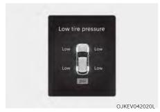
This warning message is displayed if the tire pressure is low. The corresponding tire on the vehicle illuminates.
