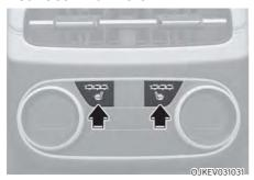
While the vehicle is on (**READY** indicator on), press the button on the center console to select the desired temperature level.
