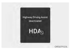
If the driver still does not have their hands on the steering wheel after the hands-off warning, 'Highway Driving Assist deactivated' warning message will appear and Highway Driving Assist and Lane Change Assist will be automatically canceled.
