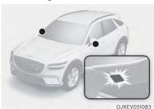
When all doors (and liftgate) are closed and locked, the puddle light will turn on for 15 seconds if the door is unlocked by the smart key or when you put your hand in the outside door handle with the smart key in possession.
