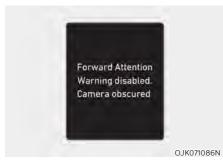
When there is an object right in front of the camera or between the driver and the camera for a certain period of time, Forward Attention Warning will not operate properly, and the 'Forward Attention Warning disabled. Camera obscured' warning message will appear on the cluster.
