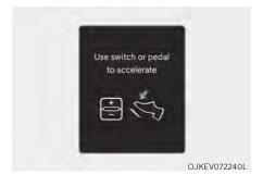
In traffic, your vehicle will stop if the vehicle ahead of you stops. Also, if the vehicle ahead of you starts moving, your vehicle will start as well. In addition, after the vehicle has stopped and a certain time have passed, the 'Use switch or pedal to accelerate' message will appear on the cluster. Depress the accelerator pedal or operate the + switch, - switch or II > switch to start driving.
