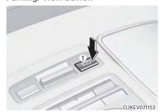
Press the Parking/View button (1) to turn on Rear View Monitor.
