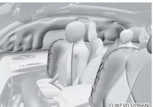
Side and curtain airbags and front center side airbag
