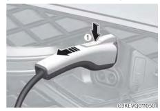
Press the release button (1), then remove the charging connector from the vehicle inlet.
