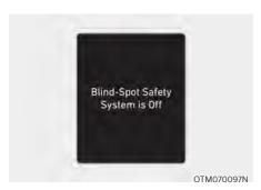
When the vehicle is restarted with Blind-Spot Collision-Avoidance Assist off, the 'Blind-Spot Safety System is Off' message will appear on the instrument cluster.
