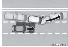
When changing lanes by detecting the lane ahead, if Blind-Spot Collision-Avoidance Assist detects that there is a collision risk with an approaching vehicle in the blind spot, it can help avoid collision by applying the brake.
