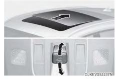
Push the sunroof switch rearward to the first detent position, the sunroof glass opens. However, if the power sunshade is closed, the power sunshade will open first.
