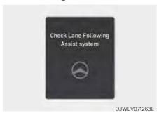
When Lane Following Assist is not working properly, the 'Check Lane Following Assist system' warning message will appear for several seconds, and the master (A) warning light will illuminate on the instrument cluster. If this occurs, have the vehicle inspected by an authorized retailer of Genesis Branded products.
