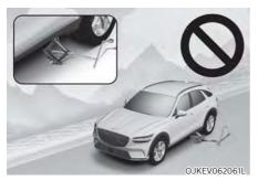
Never start or run the vehicle while an AWD vehicle is raised on a jack. The vehicle can slip or roll off of a jack causing serious injury or death to you or those nearby.
