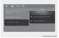
Select **Ergo-Motion Seat** from the infotainment system's Settings menu to select and set up supplemental functions for the driver.
