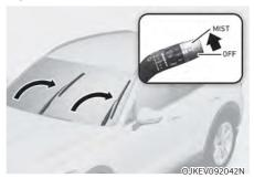
This vehicle has a "hidden" wiper design which means that the wipers cannot be lifted manually when they are in their bottom resting position.
