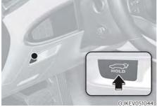
When the liftgate is closed, press the power liftgate open/close button for 1 second. The power liftgate opens or closes with a warning sound.
