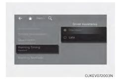
With the vehicle on, select **Setup > Vehicle > Driver Assistance > Warning Timing** from the Settings menu to change the initial warning activation time for Blind-Spot Collision-Avoidance Assist. The warning time can be set to either **Standard** or **Late**.
