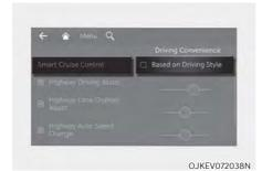
With the vehicle on, if Setup > Vehicle > Driver Assistance > Driving Convenience > Smart Cruise Control > Based on Driving Style is selected from the Settings menu, Smart Cruise Control will operate based on the driver's driving style, such as vehicle distance, acceleration, reaction speed.
