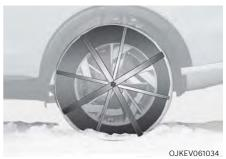
Since the sidewalls of radial tires are thinner, they can be damaged by mounting some types of snow chains on them. Therefore, the use of snow tires is recommended instead of snow chains.
