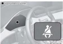
As a reminder to the driver, the seat belt warning light will illuminate for about 6 seconds each time the Start/Stop button is in the ON position regardless of belt fastening.
