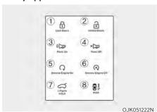
Press the icons to remotely control the vehicle.
