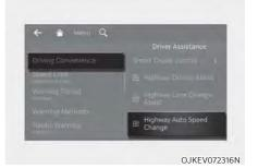
With the vehicle on, select Setup > Vehicle > Driver Assistance > Driving Convenience > Highway Auto Speed Change from the Settings menu to turn on Navigation-based Smart Cruise Control and deselect to turn off the
