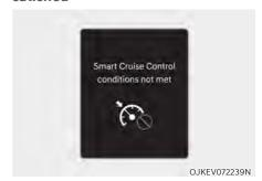
If the Driving Assist button, + switch, - switch or II S switch is pushed when Smart Cruise Control operating conditions are not satisfied, the 'Smart Cruise Control conditions not met' will appear on the cluster, and an audible warning will sound.
