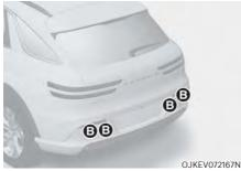
[A]: Wide-rear view camera [B]: Rear ultrasonic sensor
