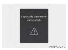
When the side view mirror warning light is not working properly, the 'Check side view mirror warning light' warning message will appear on the instrument cluster for several seconds, and the master (小) warning light will illuminate on the instrument cluster. If this occurs, have the vehicle inspected by an authorized retailer of Genesis Branded products.
