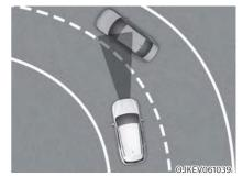
On curves, if a vehicle is detected in an adjacent lane, the regenerative braking intensity may increase and decelerate your vehicle.
