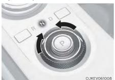
To shift the gear to N (Neutral), rotate the rotary shifter clockwise from R (Reverse) or counterclockwise from D (Drive) while depressing the brake pedal.
