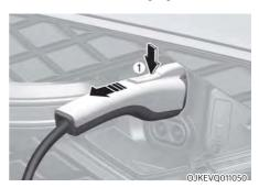
Press release button (1), then remove the charging connector from the vehicle inlet.
