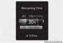
8. After charging has started, the estimated charging time is displayed on the cluster display for about 1 minute.
