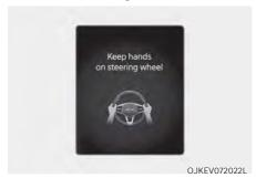
If the driver takes their hands off the steering wheel for several seconds, the 'Keep hands on steering wheel' warning message will appear on the instrument cluster, and an audible warning will sound in stages.
