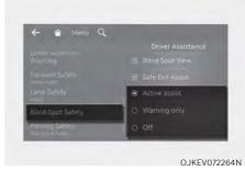
With the vehicle on, select or deselect **Setup > Vehicle > Driver Assistance > Blind-Spot Safety** from the Settings menu to set whether to use each function.
