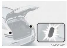
The cargo area lamp turns on when the liftgate is opened.
