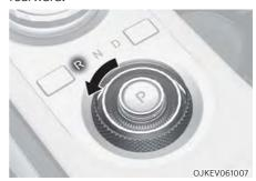
To shift the gear to R (Reverse), rotate the rotary shifter to R (Reverse) while depressing the brake pedal.
