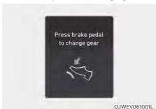
This message is displayed when the brake pedal is not depressed while shifting out of P (Park).
