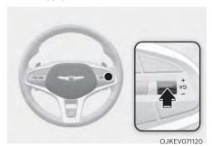
Press the **II** Switch to temporarily pause the set speed limit. The set speed limit will turn off but the Speed Limit (**O**I IMIT) indicator will stay on.
