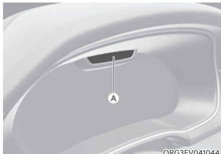
[A] : Interior view camera
