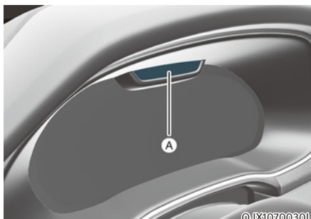
[A] : Interior view camera
