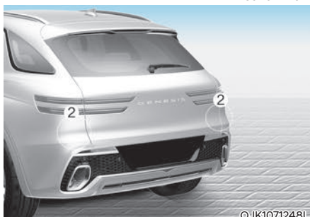
[1] : Front view camera, [2] : Rear corner radar
