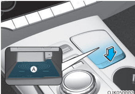
[A] : In-vehicle authentication pad (Wireless charging pad)
