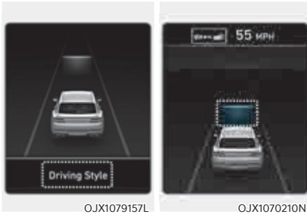
When Based on Driving Style is operating, 'Driving Style' message will appear on the cluster for 2 seconds, and the distance level and target distance will be displayed based on the driving style.
