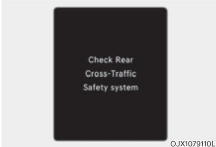
When Rear Cross-Traffic Safety system is not working properly, the 'Check Rear Cross-Traffic Safety system' warning message will appear on the cluster, and the system will turn off automatically or the system will be limited. Have the system inspected by an authorized retailer of Genesis Branded products.
