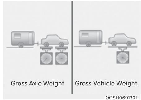
The tongue load is an important weight to measure because it affects the total Gross Vehicle Weight (GVW) of your vehicle. The trailer tongue should weigh a minimum of 10% of the total loaded trailer weight, within the limits of the maximum (15%) trailer tongue load permissible.
