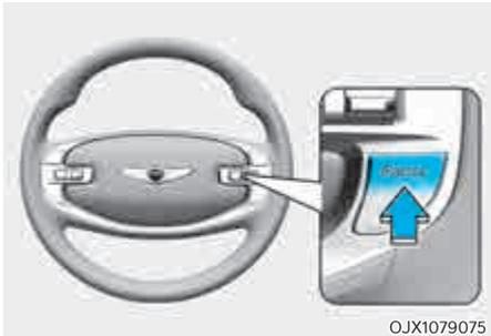
1. Press and hold Driving Assist (MODE) button at the desired speed. The Speed Limit (LIMIT) indicator will illuminate on the cluster.
