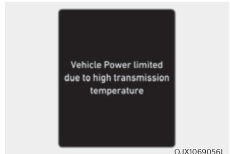
This message is displayed when the transmission oil temperature is high. Drive at steady speed or stop the vehicle at a safe place with the engine on. When the oil temperature returns to normal, the message will disappear.
