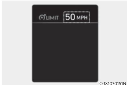
3. The set speed limit will be displayed on the cluster. If you would like to drive over the preset speed limit, depress the accelerator pedal beyond the pressure point to activate the kickdown mechanism. The set speed limit will blink and chime will sound until you return the vehicle speed within the speed limit.
