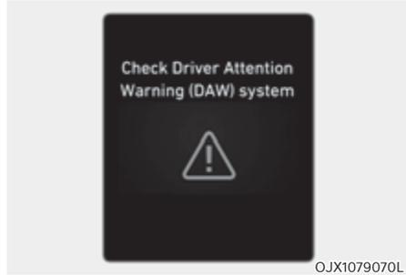
When Driver Attention Warning is not working properly, the 'Check Driver Attention Warning (DAW) system' warning message will appear on the cluster. If this occurs, have the system inspected by an authorized retailer of Genesis Branded products.
