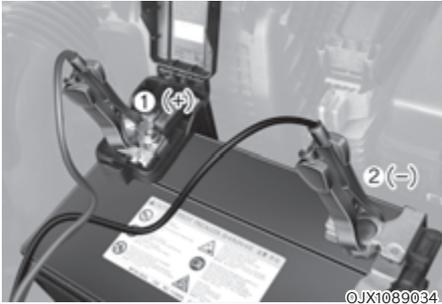
5. Connect cables (4) to the battery in numerical order.
