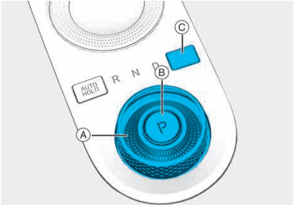
Depress the brake pedal whenever rotating the shift dial to change gear or shifting P.
