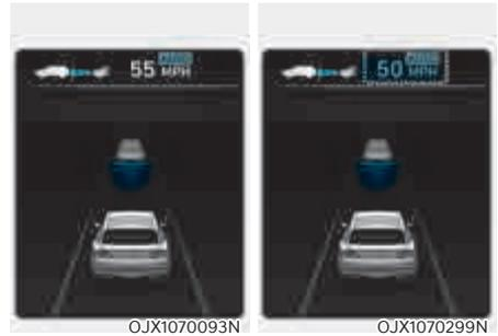
If temporary deceleration is required in the standby state and Navigation-based Smart Cruise Control is operating, the green **AUTO** symbol will illuminate on the cluster.
