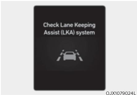
When Lane Keeping Assist is not working properly, the 'Check Lane Keeping Assist (LKA) system' warning message will appear and the yellow
