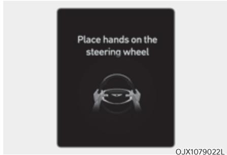
If the driver takes their hands off the steering wheel for several seconds, the 'Place hands on the steering wheel' warning message will appear and an audible warning will sound in stages.
