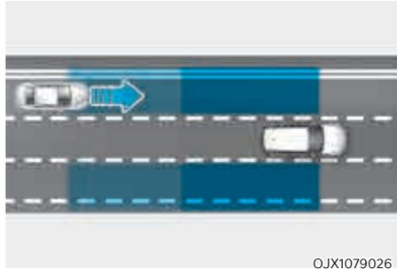
Blind-Spot Collision Assist helps detect and informs the driver that a vehicle is approaching at high speed from the blind spot area.
