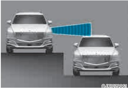
Blind-Spot Safety system may not operate properly when driving where the heights of the lanes are different. The system may not detect the vehicle on a road with different lane heights (underpass joining section, grade separated intersections, etc.). Always pay attention to road and driving conditions while driving.
