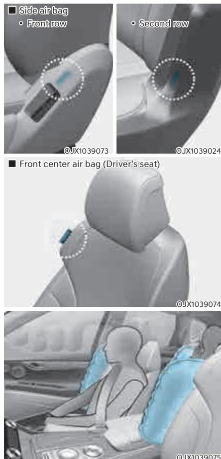
Your vehicle is equipped with a side air bag in each front and outboard second row seat. Additionally, a front center air bag is provided in the inboard side of the driver seatback. The purpose of the air bag is to provide the vehicle's additional protection than that offered by the seat belt alone.
