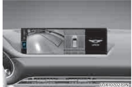
You can change Surround View Monitor settings by pressing the setup icon (⚙️) on the screen while the system is operating, or select 'Driver Assistance → Parking Safety → Camera Settings' from the Settings menu while the Engine Start/Stop button is in the ON position.
