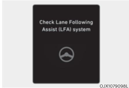
When Lane Following Assist is not working properly, the ‘Check Lane Following Assist (LFA) system’ warning message will appear on the cluster. If this occurs, have the system inspected by an authorized retailer of Genesis Branded products.
