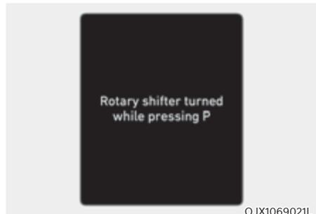
This message is displayed when the shift dial is rotated while pressing the P button.
