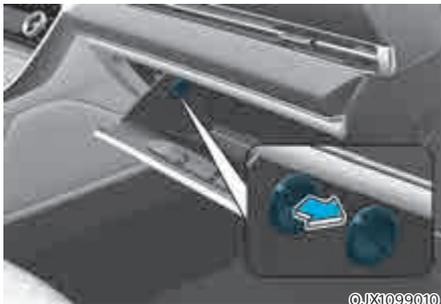
2. Remove the stoppers on both sides to allow the glove box to hang freely on the hinges.
