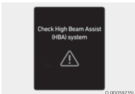
When High Beam Assist is not working properly, the 'Check High Beam Assist (HBA) system' warning message will appear and a warning light will illuminate on the cluster. Have the system inspected by an authorized retailer of Genesis Branded products.
