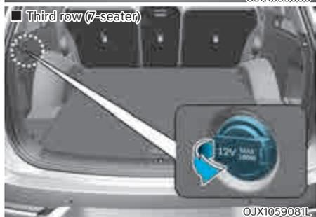
The power outlet is designed to provide power for mobile telephones or other devices designed to operate with vehicle electrical systems. The devices should draw less than 180 watts with the engine running.
