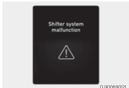
This message is displayed when the transmission or the shift button does not properly operate in the P (Park) position. Immediately have the vehicle inspected by an authorized retailer of Genesis Branded products.
