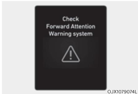
When Forward Attention Warning is not working properly, the 'Check Forward Attention Warning system' warning message will appear on the cluster. If this occurs, have the system inspected by an authorized retailer of Genesis Branded products.
