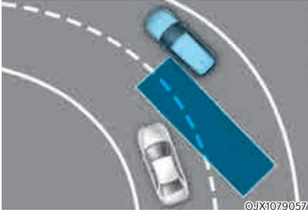
Blind-Spot Safety system may not operate properly when driving on a curved road. The system may not detect the vehicle in the next lane.
