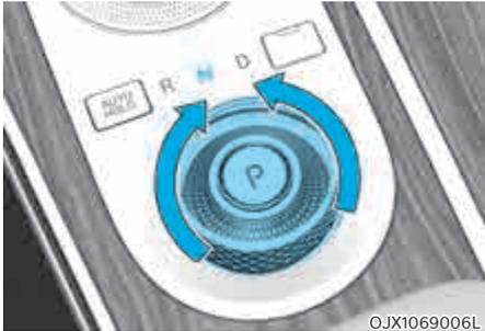
To shift the gear to N (Neutral), rotate the shift dial clockwise from R (Reverse) or counterclockwise from D (Drive) while depressing the brake pedal.
