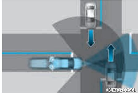
Junction Crossing function will help avoid a collision with oncoming vehicles on the left or right side when crossing an intersection by applying emergency braking.
