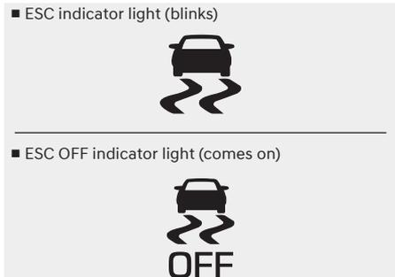
When the Engine Start/Stop button is pressed to the ON position, the ESC indicator light illuminates, then goes off if the ESC system is operating normally.
