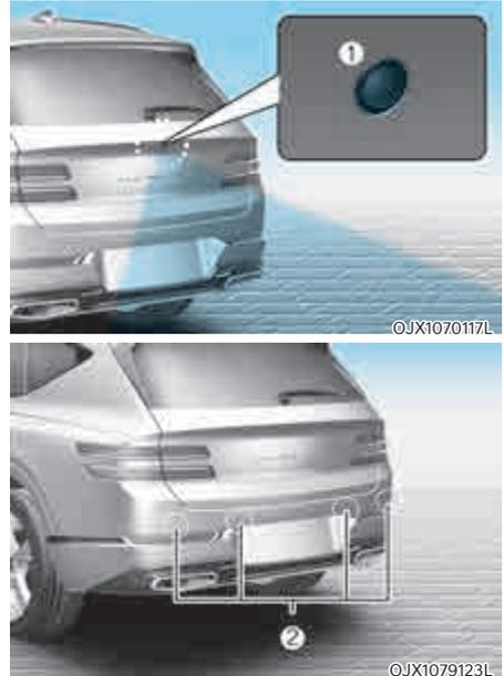
[1]: Rear view camera, [2]: Rear ultrasonic sensors
