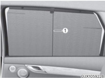
If excessive force is applied on the antenna rod (1), the sunshade may deform and malfunction.
