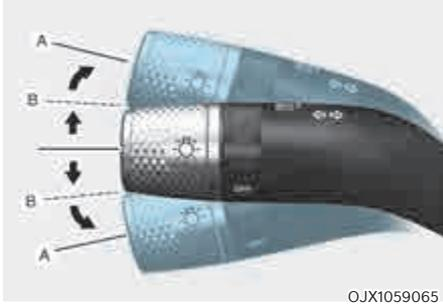
To signal a turn, push down on the lever for a left turn or up for a right turn in position (A).
