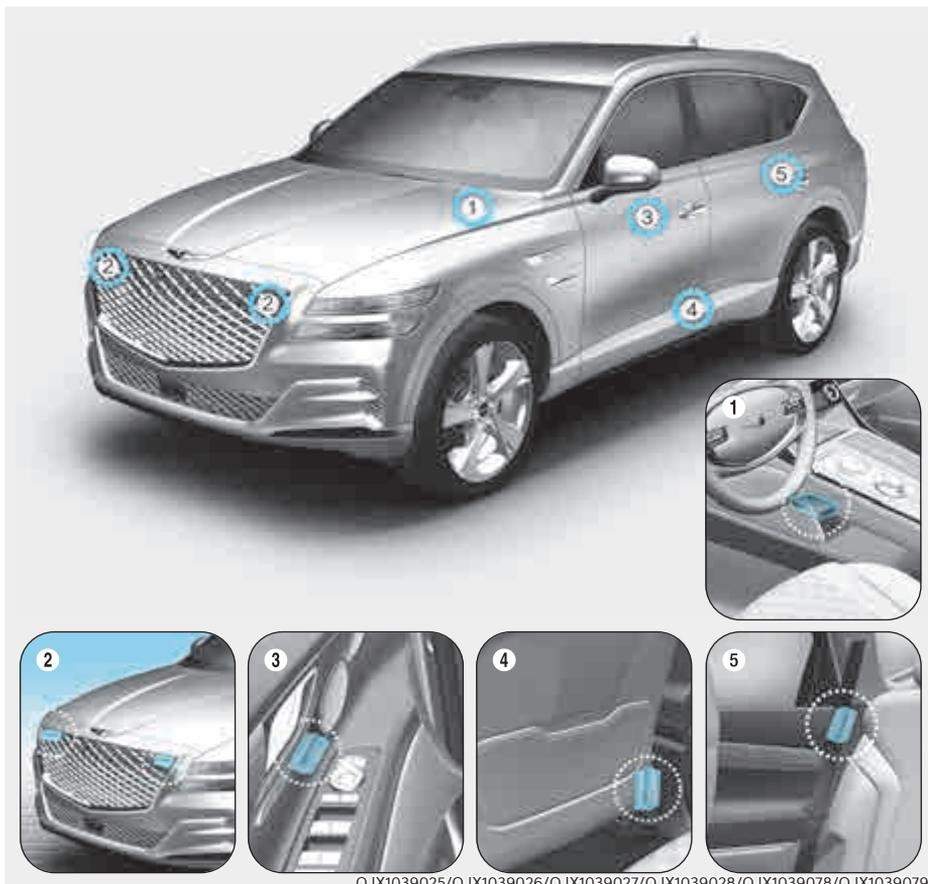
1. SRS control module / Rollover sensor
