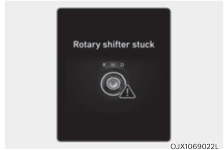
This message is displayed when the shift dial does not return back to its normal position after rotating it. Immediately have the vehicle inspected by an authorized retailer of Genesis Branded products.
