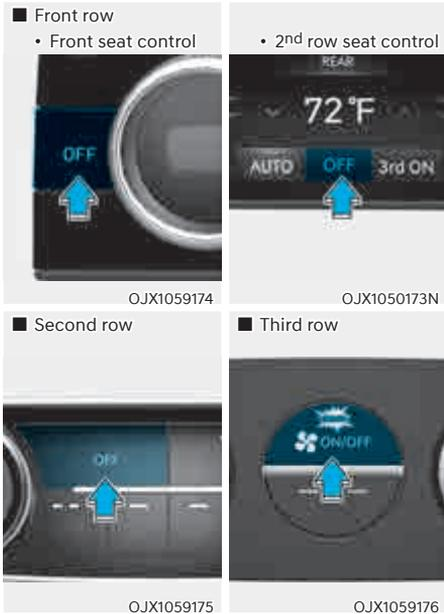
Touch the OFF icon or press the OFF button to turn the climate control system off. You can still operate the mode and air intake buttons as long as the Engine Start/Stop button is in the ON position.
