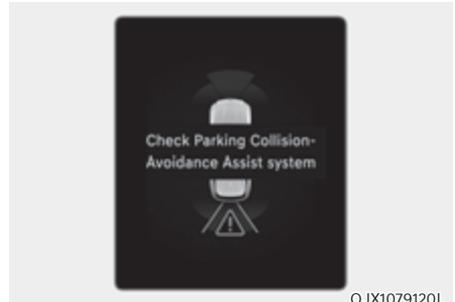
When Reverse Parking Collision-Avoidance Assist or other related systems are not working properly, the 'Check Parking Collision-Avoidance Assist system' warning message will appear on the cluster, and the system will turn off automatically. Have the system inspected by an authorized retailer of Genesis Branded products.
