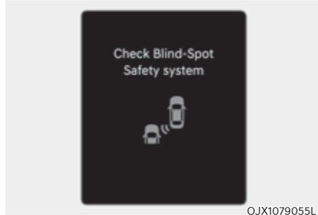
When Blind-Spot Safety system is not working properly, the 'Check Blind-Spot Safety system' warning message will appear on the cluster, and the system will turn off automatically or the system will be limited. Have the system inspected by an authorized retailer of Genesis Branded products.
