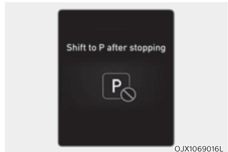
This message is displayed when the gear is shifted to P (Park) while the vehicle is moving.
