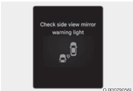
When the side view mirror warning light is not working properly, the 'Check side view mirror warning light' warning message will appear on the cluster. Have the system inspected by an authorized retailer of Genesis Branded products.
