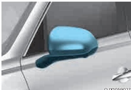
Your vehicle is equipped with both left-hand and right-hand side view mirrors. The mirrors can be adjusted with the mirror adjustment control switch. The side view mirrors can be folded to help prevent damage when going through an automatic car wash or when passing through a narrow street.
