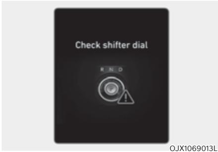
This message is displayed when there is a malfunction with the shift dial. Immediately have the vehicle inspected by an authorized retailer of Genesis Branded products.
