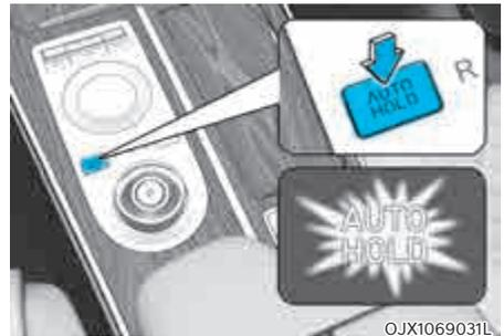
1. With the driver's door and engine hood closed, depress the brake pedal and then press the AUTO HOLD switch. The white AUTO HOLD indicator will come on and the system will be in the standby position.
