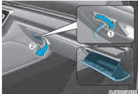
The glove box can be locked and unlocked with the mechanical key (1).
