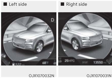
Blind-Spot View Monitor displays the rear blind spot area of the vehicle in the cluster when the turn signal is turned on to help change lanes.
