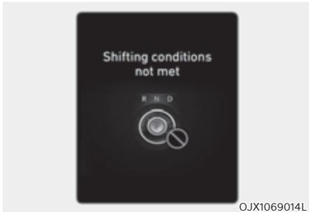
This message is displayed when engine RPM is too high, or when driving speed is too fast to shift the gear. Decrease vehicle speed or slow down before shifting the gear.
