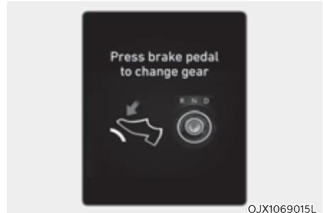
This message is displayed when the brake pedal is not depressed while shifting the gear.
