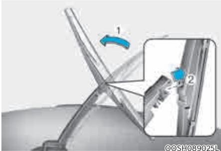
1. Raise the wiper arm and then rotate the wiper blade assembly (1).
