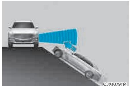
Rear Cross-Traffic Safety system may be limited when the vehicle is on an uphill or downhill slope, or near it, and may not detect the vehicle approaching from the left or right. If this occurs, the system may not warn the driver or control the brakes when necessary.
