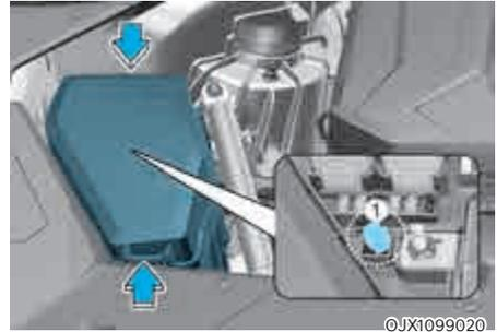
5. Pull the suspected fuse straight out. Use the removal tool (1) provided in the engine compartment fuses panel cover.
