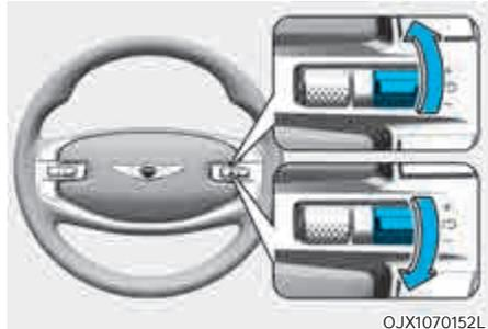
2. Push the + switch up or - switch down, and release it at the desired speed. Push the + switch up or - switch down and hold it. The speed will increase or decrease to the nearest multiple of five (multiple of ten in km/h) at first, and then increase or decrease by 5 mph (10 km/h).
