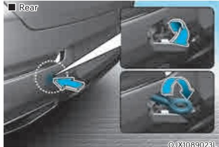
2. Remove the hole cover by pressing the lower part of the cover on the bumper.
