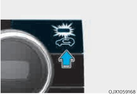
The air intake control button is used to select either Fresh mode (outside air) or Recirculation mode (cabin air).
