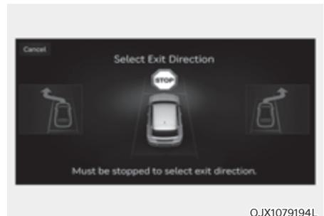
With the vehicle stopped by depressing the brake pedal, touch the infotainment system screen or use the central controller to select the desired exit direction.
