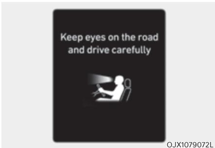
Forward Attention Warning helps determine whether the driver is focused on the road depending on information, such as the amount of time the driver is looking elsewhere, the amount of time the eyes are closed, how frequently the driver yawns, etc. If the system judges the driver is not focused, the 'Keep eyes on the road and drive careful' warning message will appear on the cluster, and an audible warning will sound.
