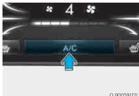
Touch the A/C icon to manually turn the air conditioning on (indicator light will illuminate) and off.
