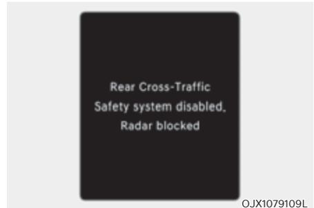
When the rear bumper around the rear-side radar or sensor is covered with foreign material, such as snow or rain, or installing a trailer or carrier, it can reduce the detecting performance and temporarily limit or disable Rear Cross-Traffic Safety system.
