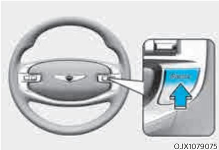
Press the Driving Assist
