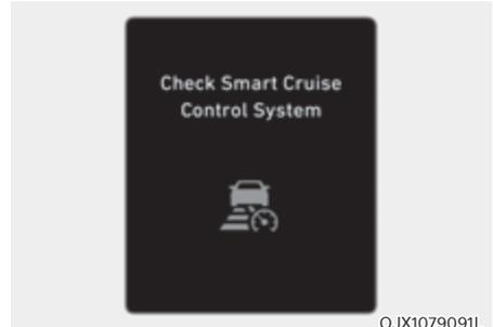
When Smart Cruise Control is not working properly, the 'Check Smart Cruise Control system' warning message will appear, and the
