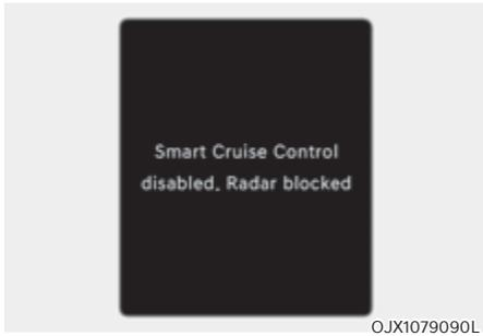
When the front radar cover or sensor is covered with snow, rain, or foreign material, it can reduce the detecting performance and temporarily limit or disable Smart Cruise Control.
