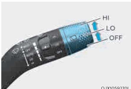
The rear window wiper and washer switch is located at the end of the wiper and washer switch lever. Turn the switch to the desired position to operate the rear wiper and washer.
