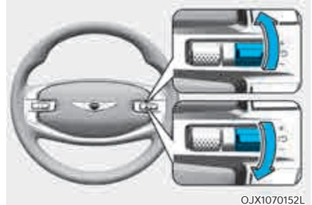
To resume Manual Speed Limit Assist after the system was paused, push the +, -,
