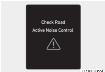
When Road Active Noise Control is not working properly, this warning message will appear on the cluster LCD display. If this occurs, have the system inspected by an authorized retailer of Genesis Branded products.
