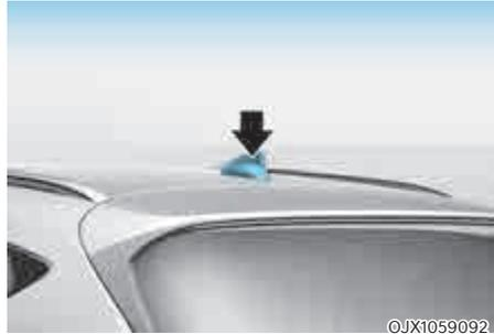
The shark fin antenna will receive AM, FM broadcast and SXM channel signals and transmit data.
