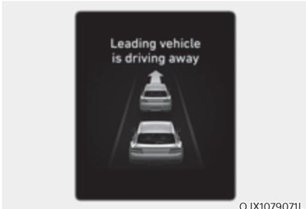
When the front vehicle departs from a stop, Leading Vehicle Departure Alert will inform the driver by displaying the 'Leading vehicle is driving away' message on the cluster and an audible warning will sound.
