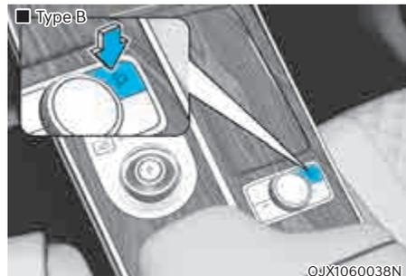
Downhill Brake Control assists the driver to descend down a steep hill without having to depress the brake pedal.
