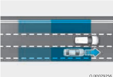
Blind-Spot Collision-Avoidance Assist will help detect and inform the driver that a vehicle is in the blind spot.
