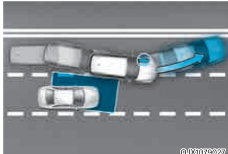
When changing lanes by detecting the lane ahead, if the system judges that there is a collision risk with an approaching vehicle in the blind spot, the system will help avoid a collision by applying the brake.
