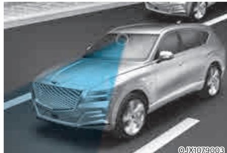
The front view camera is a sensor that detects the front road. If the windshield or the front view camera is covered with snow, rain or foreign matters, the data collected by the camera is limited due to the degradation of the camera's performance. Always keep the front view camera clean.
