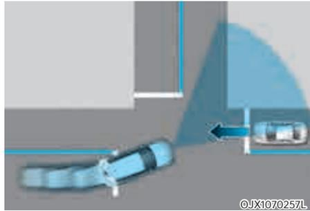
Junction Turning function will help avoid a collision with an oncoming vehicle in an adjacent lane when turning left at a crossroad with the turn signal on by applying emergency braking.
