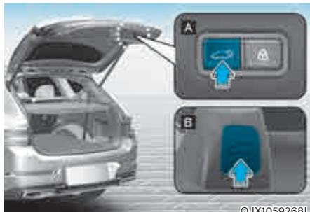
If the battery has been discharged or disconnected, or if the power liftgate fuse has been replaced or removed, reset the power liftgate by performing the following procedure:
