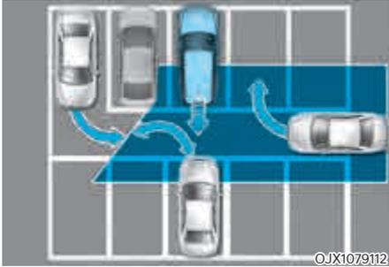
Rear Cross-Traffic Safety system may detect vehicles which are parking or pulling out near your vehicle (for example: a vehicle leaving beside your vehicle, a vehicle parking or pulling out in the rear area, a vehicle approaching your vehicle making a turn, etc.). If this occurs, the system may unnecessarily warn the driver and control the brake.
