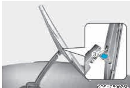
3. Install the new blade assembly by inserting the center part into the slot in the wiper arm until it clicks into place (3).
