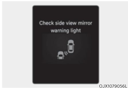
When the side view mirror warning light is not working properly, the 'Check side view mirror warning light' warning message will appear on the cluster. Have the system inspected by an authorized retailer of Genesis Branded products.
