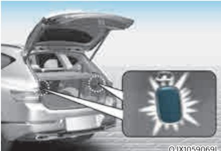
The lamp turns on when the liftgate is opened.
