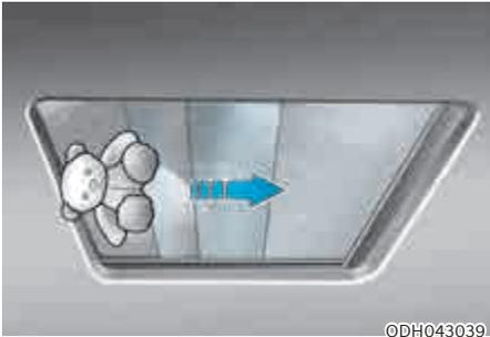
If the sunroof senses any obstacle while it is closing automatically, it will reverse direction then stop to allow the object to be cleared.
