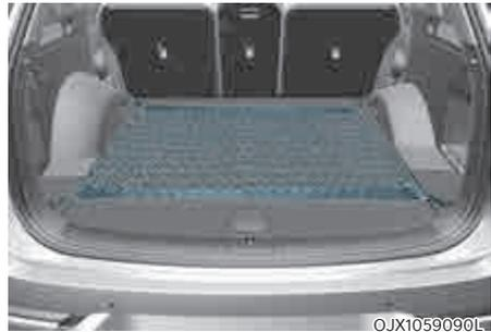
To keep items from shifting in the cargo area, you can use the 4 holders located in the luggage board to attach a cargo net.
