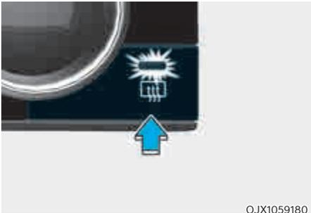
The defroster heats the window to remove frost, fog and thin ice from the interior and exterior of the rear window, while the engine is running.
