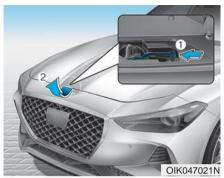
3. Raise the hood slightly, push the secondary latch up (1) inside of the hood center and lift the hood (2). After it has been raised about halfway, it will raise completely by itself.
