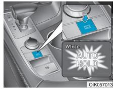
With the driver's door, engine hood and trunk closed, fasten the driver's seat belt or depress the brake pedal and then press the [AUTO HOLD] switch. The white AUTO HOLD indicator will come on and the system will be in the standby position.
