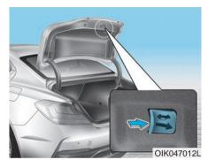
Your vehicle is equipped with an Emergency Trunk Safety Release lever located inside the trunk. When someone is inadvertently locked in the trunk, the trunk can be opened by moving the lever in the direction of the arrow and pushing the trunk open.
