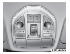
The Engine Start/Stop button must be in the ON or START position before you can open or close the sunroof.
