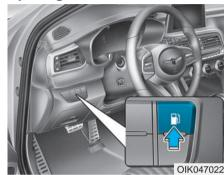
The fuel filler door must be opened from inside the vehicle by pushing the fuel filler door opener button.
