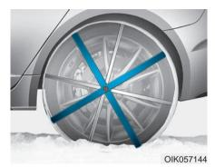
Since the sidewalls on some radial tires are thinner than other types of tires, they may be damaged by mounting certain types of tire chains on them. Do not mount tire chains on vehicles equipped with aluminum wheels: unavoidable use AutoSock® (fabric snow chain or similar). Install the tire chain after reviewing the instructions provided with the tire chains. Damage to your vehicle caused by improper tire chain use is not covered by your vehicle manufacturer's warrantv.
