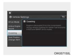
Select 'Settings  $\rightarrow$  Vehicle settings  $\rightarrow$  Coasting' on the audio or AVN screen. Turn the function ON and the ECO Coasting function will activate.
