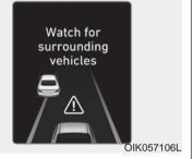
If the vehicle ahead (vehicle speed: less than 20 mph (30 km/h)) disappears to the next lane, the warning chime will sound and a message "Watch for surrounding vehicles" will appear. Adjust your vehicle speed for vehicles or objects that can suddenly appear in front of you by depressing the brake pedal.
