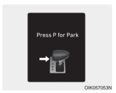
The message appears on the LCD display to inform the driver to press the P button to shift to P (Park) when the driver moves the shift lever upward even though the gear is in R (Reverse).
