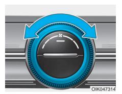
The fan speed can be set as desired by turning the fan speed control knob. Turn the knob to the right for higher fan speed.
