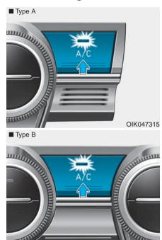
Push the A/C button to manually turn the system on (indicator light will illuminate) and off.
