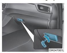
When leaving keys with parking lot and valet attendants, the following procedures will ensure your vehicle's glove box compartment can only be opened with the mechanical key.
