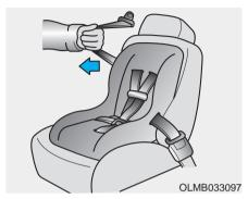
3. Pull the shoulder portion of the seat belt all the way out. When the shoulder portion of the seat belt is fully extended, it will shift the retractor to the "Automatic Locking" (child restraint) mode.
