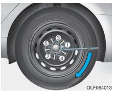
13. Use the wheel lug nut wrench to tighten the lug nuts in the order shown. Double-check each lug nut until they are tight. After changing tires, have an authorized retailer of Genesis Branded products tighten the lug nuts to their proper torque as soon as possible. The wheel lug nut should be tightened to 79~94 lbf-ft (11~13 kgf-m).
