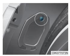
Remove the service cover (1) under the wheel housing by pushing out the retainer clip with a slim tool. If it is difficult to remove the service cover because of the tire, steer the tire inward.
