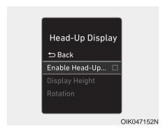
To activate the head up display, select 'Head-UP Display' on the User Settings mode on the instrument cluster LCD display.
