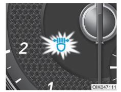
If the AFS malfunction indicator comes on, the AFS is not working properly. Drive to the nearest safe location and restart the engine. If the indicator continuously remains on, have the system checked by an authorized retailer of Genesis Branded products.
