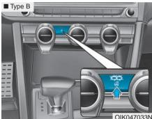
When the Engine Start/Stop button is in the ON position, press the heated steering wheel switch to warm the steering wheel.
