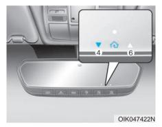
If the both indicator (4) and (6) are flashing rapidly for about 5 seconds, the two way synchronization is completed.
