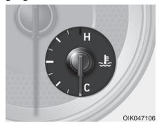
This gauge indicates the temperature of the engine coolant when the Engine Start/Stop button is in the START position.
