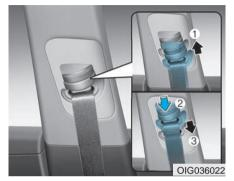
To adjust the height of the seat belt anchor, lower or raise the height adjuster into an appropriate position.
