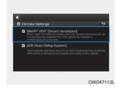
The smart ventilation system helps maintain pleasant/fresh air condition inside the passenger compartment by automatically detecting/controlling the temperature, humidity, etc., when you drive the vehicle with the climate control system in the OFF position. When the smart ventilation system starts to operate, the message, "SMART VENTILATION ON" appears for 5 seconds.
