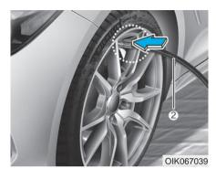
Unscrew the valve cap from the valve of the flat tire and screw the filling hose (2) of the sealant bottle onto the valve.
