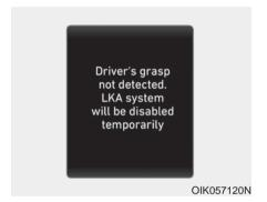
If the driver still does not have their hands on the steering wheel after the message "Keep hands on steering wheel", the system will not control the steering wheel and warn the driver only when the driver crosses the lane markers.
