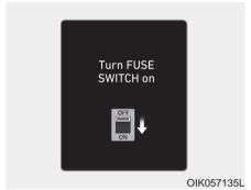
If the fuse switch is OFF, "Turn FUSE SWITCH on" message will appear.
