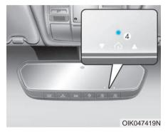
Press the Original Transmitter (OT) button until the indicator (4) is turned continuously ON or flashes in Green for approximately 10 seconds and it indicates the programing is completed.
