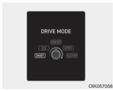
The mode changes whenever the DRIVE MODE selection knob is rotated.
