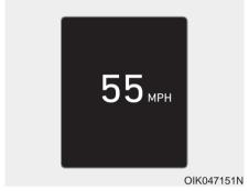
This digital speedometer display shows the speed of the vehicle.
