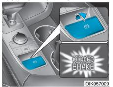
To apply the EPB (Electronic Parking Brake):
