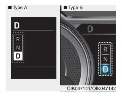
Shift indicator pop-up (if equipped) The pop-up indicates the current gear position displayed in the cluster for about 2 seconds when shifting into other positions (P/R/N/D).
