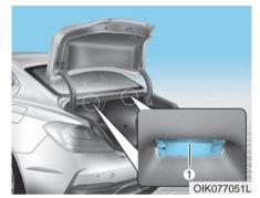
If the trunk lamp (LED) (1), does not operate, have the system be checked by an authorized retailer of Genesis Branded products.
