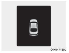
This warning is displayed if you turn off the engine when any window is open.
