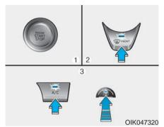
To reduce the probability of fogging up the inside of the windshield, the air intake or air conditioning are controlled automatically according to certain conditions such as or positions. To cancel or reset the defogging logic, do the following.
