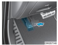
Check whether the stroke is within specification when the parking brake pedal is depressed with 44 lb (20 kg, 196 N) of force. Also, the parking brake alone should securely hold the vehicle on a fairly steep grade. If the stroke is more or less than specified, have the parking brake adjusted by an authorized retailer of Genesis Branded products.
