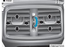
The outlet vents can be opened ( $\circledast$ ) or closed ( $\bigcirc$ ) separately using the thumbwheel.
