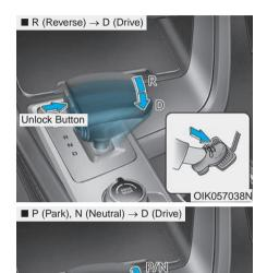
To shift into D (Drive), depress the brake pedal and press the UNLOCK button on the shift lever. Move the
