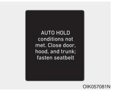
AUTO HOLD conditions not met. Close door, hood, and trunk; fasten seatbelt
