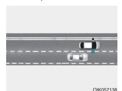
The Blind-Spot Collision Warning (BCW) range varies relative to vehicle speed. Note that if your vehicle is traveling much faster than the vehicles around you, the warning will not occur.
