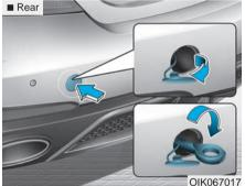
Remove the hole cover pressing the lower part of the cover on the front or rear bumper.
