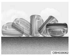
Front air bags may not inflate in rollover accidents because air bag deployment could not provide protection to the occupants.
