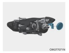
Disconnect the bulb socket-connector.
